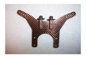
D2) Install the tower, with body mounts forward, using four 4-40 X ½" cap head bolts (two from bag, two from instruction #21). In a few bulkheads these screws have stripped when over-tightened, so don't be a gorilla here. Prototype tower in this photo, has no body mounts.
