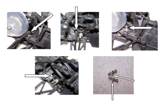
13) From the outside end of the front of the rear control arm, remove the little 2-56 screw that holds in the hub carrier. Don't lose it! Now, from the rear of the control arm, use your wrench to push the hinge pin forward so you can remove the pin. The hub carrier, with camber link and CVD assembled, will fall off. Save the spacers. Set all these parts, hub carrier assembly, hinge pin, spacer(s) and little screw, aside for re-use.
