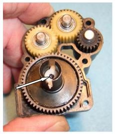
A8) In the right side of the transmission case, insert the remaining 3/8 X 3/16 bearing (6906) in the top shaft boss and the remaining outdrive bearing (6903) in its boss. Place a small bead of inexpensive grease around the mating surface of the right transmission half. This grease only helps keep dirt out, it does not lubricate anything. Grease attracts dirt; paradoxically this grease is used to seal out dirt, so be thorough, but don't use more than is needed. A little touch means so much.
