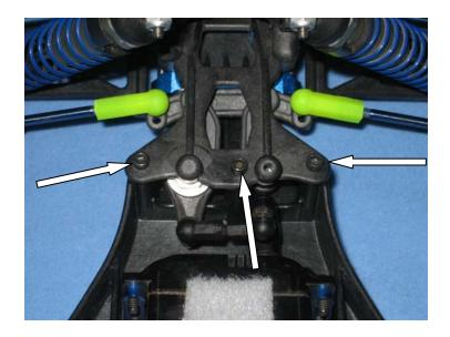
A16) Carefully turn the chassis & front suspension over. Install the two 5/8" flat head screws you removed from the bulkhead back into the rear-most of the four holes at the front of the chassis.
