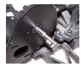
17) From under the truck remove the two flat head screws that hold the motor guard. Then, from above, remove the two button head screws that hold the motor guard to the top rear of the transmission. The motor guard and the two button head screws will not be needed. Save one flat head screw for re-use in B-11.
