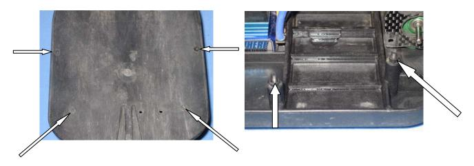
A14) Position the T4 front suspension and steering over the front of the chassis just as it was on your T4. Be careful that the steering assembly remains in place and that the bulkhead (9563) stays in position with the top plate (9566). The top plate should fit snugly over the center post in the chassis and on the bosses at each side of the front of the chassis.
