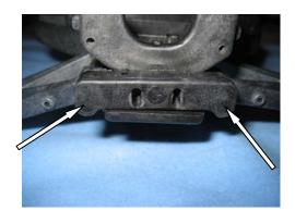
C10) Secure the toe-in bar with two 4-40 X 3/4" cap head screws and flat washers (small arrows). Leave the screws finger-tight for now. The bar must be free to move up and down in its slots and there should be a gap between the bar and the chassis (large arrow).
