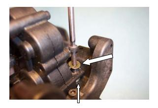
B10) Place the final spacer under the left front transmission mounting tab. Put the washer on the 4-40 X ½" button head bolt and engage the bolt with your wrench. Work the wrench down between the transmission and the motor plate to install this screw. Be careful not to strip the threads in the insert. When the left front bolt is properly engaged in its insert, apply final torque to all four transmission
