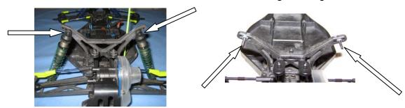
10) Remove the nuts that hold the shock bolts in the tower. Remove the bolts, and save the bolts, nuts, bushings and plastic nuts for re-use.
