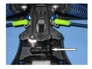
D6) Install the motor using the two motor screws from your T4.
