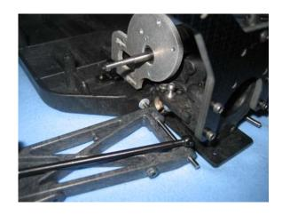
C9) Your X – 60 has been supplied with two toe-in bars, 3 degrees and 4 degrees. Check the Tuning Section and Set-Up sheets to determine which you will use. Engage the rear of the hinge pins in their holes in the toe-in bar. The bar will extend across the back of the chassis.
