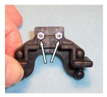
B4) Turn the chassis upside down and mate the bulkhead to the chassis. Take care that the threaded inserts remain in their hexes in the bulkhead and go into their hexes in the chassis. This is a pain to do, but most likely you'll only have to do it once. When you've got it right, secure the bulkhead by finishing installation of the 5/8" cap head from B3 above.
