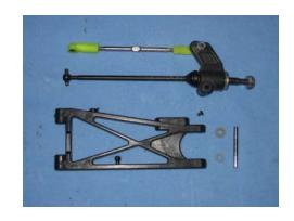
C2) Check the Tuning Section and Set-Up sheets for hub spacing. These instructions show hub in the center. Slide the hinge pin in from the rear, add one spacer (4187), then start the pin through the hub carrier.
