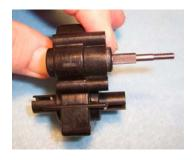
A10) Install the 4-40 X 3/8" bolt in the corner (short arrow) and the 4-40 X ½" bolt (from instruction #22) in the rear center of the transmission (long arrow). Leave them finger tight until step A12. Make sure the head of the 3/8" bolt is fully down in its boss and no part of the bolt protrudes on either side. This part of the transmission must fit into the "box" at the rear of the chassis.
