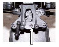
7) Remove the two side top plate screws. Save them for re-use. Carefully remove the front end and steering assembly, and set it aside for re-use. Make sure the steering linkage stays in place.
