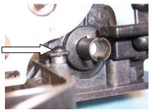
B11) Install the ½" flat head (from instruction #17) through the motor plate and motor plate support. You may need to loosen the two bolts that hold the support in the car. Secure with the flat washer and lock nut. Remember to re-tighten the motor plate support bolts when this step is finished. Some drivers foolishly leave this bolt out, but it is very important to prevent chassis flex and bending the motor plate.
