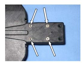
B2) Install the motor plate support bracket using two 4-40 X ¼" flat head screws. The screws come up from underneath the chassis and thread into the support. Notice the support is off-set to the left.
