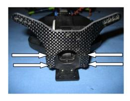
D3) Install the rear shocks to the front of the shock tower and the rear of the control arms using all the parts saved from your T4. This photo still has a prototype body mount.
