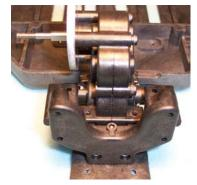
B7) Remove the transmission from the truck. Check the Tuning Section and Set-Up sheets to determine how high you will mount your transmission and select the proper shims from the bag of shims. Assemble three 4-40 X 5/8" cap head bolts, one 4-40 X ½" button head bolt, four flat washers, and the shims. Note that the short button head screw will be at the left front (arrow).
