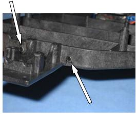
C7) Place the Lunsford Ti hinge pins in the two rear control arms. Insert the front end of the hinge pins into the bushings. Check the Tuning Section and Set-Up sheets. Here we have placed spacers in front of the arms and behind them.
