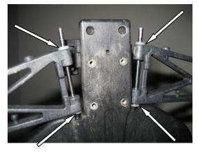
C8) X – 60 control arms and toe-in bars have been designed for about .060" of shims. Your AE shims are about .030, so the arms can go forward, middle, or back. Team drivers rarely space the arms forward, and they like having a shim between the arm and the bushing.
