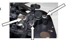
20) Two flat head screws hold the body mounts on from the front of the tower. You may remove them and the mounts if you wish, or just loosen and twist the mounts out of the way for step 21.
