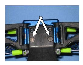
A17) Place the front bumper (9562) in position and secure it with the two 5/8" flat head screws you took out.
