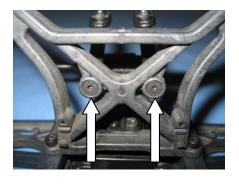
21) From the top, put your wrench down between the body mounts and remove the two cap head screws that secure the transmission to the shock tower. You should now be able to remove the transmission from the truck. Save the screws for re-use in D-2.
