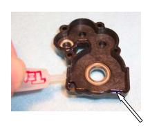
A9) Some Team drivers put a small amount of AE Stealth Lube on the teeth of their diff gear to lubricate the transmission. Other Team drivers do not, saying the trans is freer without the grease. Pay your money and take your pick. Carefully put the two halves of the transmission together. Make sure everything rotates very freely. Later is not the time to repair a binding transmission. Wipe excess grease off the outside of the case.
