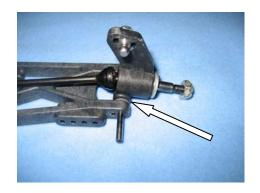
C3) Place the second spacer (4187) between the hub carrier and the front of the control arm and slide the hinge pin the rest of the way through.
