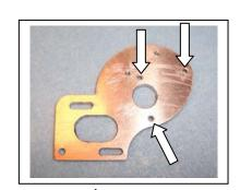
A12) Insert the three 4-40 X 1" screws (from instruction #19) through the transmission case, threading them into the motor plate finger tight. Check once again to ensure the transmission rotates freely but without excessive slop. This is your last chance! Now put the final torque on all five transmission bolts.
