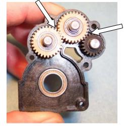
A7) Insert the diff through the outdrivebearing in the left transmission case half. The head of the diff screw should be up (arrow). Make sure all the gears are properly meshed and the trans rotates freely.
