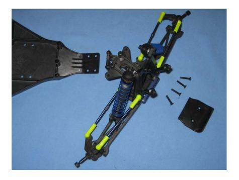
A15) Secure the top plate with the three screws you took out from the T4. Leave these screws finger-tight for now.
