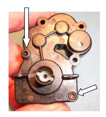
A11) The motor plate has two extra 4-40 tapped holes which are useful to install a fan for the motor (left photo). The arrows in the right photo point to the three holes that attach the plate to the transmission. Team drivers put a drop of thread lock in these holes prior to the next step. Thread lock on the long bolts will come off going through the transmission, so a drop here works best.
