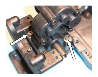
B9) Place a flat washer about half way on the last 4-40 X 5/8" cap head bolt. Slide the spacer under the right rear transmission mounting tab (small arrow). Put the bolt in so the washer is beneath the transmission case bolt (large arrow), then install the bolt finger tight. The head of this bolt will rub on the case bolt a bit, but that's OK.
