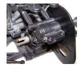
18) Remove the long bolt through the transmission that holds the body mounts. This bolt will not be needed.
