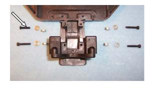
B8) Place the shims for the left rear and right front transmission bolts on their chassis bosses. Slide the transmission down over
