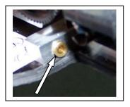
E10) Place the hinge pins (XF6141) into the bushings.
