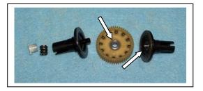
A3) Remove the 12 diff balls (XF6500) and bearing from the gear (AE7664). Clean the balls and gear and set them aside to air dry. Clean and re-lube the two diff bearings, using just a drop of good bearing oil. Set the spring and T-nut aside with the gear, balls, and bearings. This leaves the outdrives in front of you. Remove the diff rings and clean them. Our second diff bearing wanted to stay in the outdrive, so we removed it
