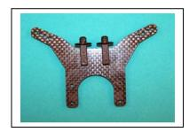
G2) Install the tower to the back of the bulkhead using four 4-40 X 1/2" cap head bolts (two from bag G and two from Inst 13 and four flat washers.
