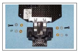
D8) Place the four shims on the four posts of the cradle and put the transmission into the cradle. Be sure the shims stay in place (bottom photo) and the motor plate lines up correctly with its bracket (right photo).
