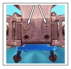
From the top, remove the center screw that holds the top plate to the chassis post. (Left photo) Then remove the two side screws. (Right photo) Save the screws for re-use. This truck had cap head screws with flat washers, yours may be different.
