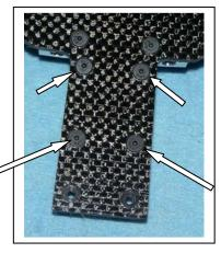
D3) Now install the transmission cradle (XF5030). If you use thread lock, do only the two front holes. The two rear holes are not tapped, but you will want to twist the 1" bolts to help the cradle slide down. You want to twist a little bit on each bolt in order to keep the cradle level as you install it. "Walk" it down. Don't let it get on a large angle as in the left and center photos. Keep it level, as in the right photo.
