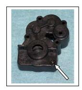
A22) The X Factory 4-Gear motor plate (XF1232) has two "extra" holes (left photo) which are useful to install the optional ES008 heatsink and fan. Arrows in the right photo point to the three holes that attach the motor plate to the transmission. Team drivers put a drop of threadlock now in these three holes. Don't put the threadlock on the bolts as it will come off
