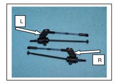
E4) Let's do the left arm first. Check the set-up sheet and tuning section to determine whether you will mount the hubs rear, middle, or forward. Here we show the middle position. Begin sliding the hinge pin through the outer end of the control arm, and place one shim on the pin.
