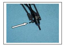
E6) Put another spacer between the hub carrier and the arm, then slide the pin the rest of the way through.
