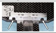
D2) Put two 4-40 X 1" flat head bolts (XF6027 long arrows) and two 4-40 X 3/8" flat head bolts (short arrows) up from the bottom of the chassis to bolt on the transmission cradle. 1" bolts to the rear, 3/8" to the front. The very back chassis holes will be used later.
