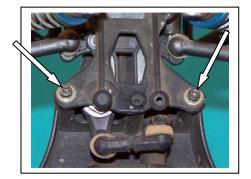
7) Carefully remove the front suspension and steering assembly and set it aside for re-use. Make sure the steering linkage stays in place.
