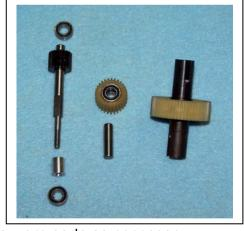
& two 3/16 X 3/8 bearings (XF6200). Replace worn parts as necessary.
