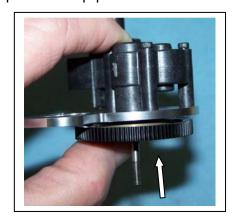
A26) Turn the transmission back over so the top shaft is pointing up, but be certain the slipper pad remains engaged in the spur and the spur is tight against the plate. Put the second slipper pad in its place on the spur and slide the second slipper plate, flat side down, onto the shaft.
