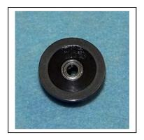
A7) Install the spring and T-nut into the male outdrive. Be certain the lugs on the T-nut engage properly in the slots of the outdrive. Set aside until A10.
