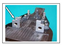
C3) Use two 4-40 X 3/8" cap head screws (short arrows) to attach the back of the front decks (XF1500) to the notch part of the support brackets. The front hole should line up with the stand-offs. (long arrows) Only finger-tight for now.
