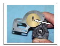
A25) Put a slipper pad (AE9603) on the 78 tooth spur gear (AE9652) supplied in your Kit – the larger one from the T 4.1 will not fit. (left & center photos). The hex of the pad fits into the molded hex in the gear. Now turn the transmission so the top shaft with slipper plate is facing down. Hold the plate on with your thumb and slide the spur gear, pad side up, onto the shaft so the pad & gear are tight against the plate. Keep pressure on the
