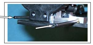
E11) Check the set-up sheet and tuning section to determine whether your control arm inner pivot will be forward, center, or rear. Here we are using arms rear, so the shims go on the front. We use some extra 0.090" transmission shims; shock limiters, flat washers, almost any shim of the correct size will do. If your set-up is arms back, slide the shims on the hinge pins now.
