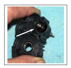
A16) Gather together the idler gear from the T 4.1 (AE9360) along with its 3/16" X 3/8" bearings (XF6202) and shaft (XF5201) along with the same parts from bag A so you have two gears, two shafts, and four bearings. Install a bearing into each side of both idler gears. Team drivers do it by pushing on the outer race with a socket.
