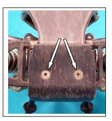
5) Still working beneath the chassis, remove the two flat head screws which hold the bulkhead to the chassis. Save these screws for re-use.
