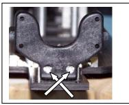
D7) Gather together two 4-40 X 3/8" cap head screws, two 4-40 mini nuts (XF6073), and four #4 flat washers (XF6080). Check the tuning section and set-up sheet to determine which transmission shims (XF5702) you will use, get those four shims out of the bag, and save the others. Here we are using the 0.060" shims.
