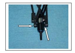
E7) Install the 2-56 X 1/8" button head screw to secure the hinge pin. (Now where did you put that little thing???)
