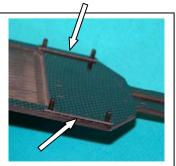
F2) If you use it, place a drop of thread lock in the two holes of each rear top deck support (XF1311) and install them on each side of the chassis.
