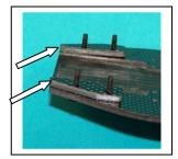
B3) Place the nose bridges (XF 1530 long arrows) over the spacers & screws and secure with locking nuts (XF6071 short arrows).
