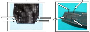
B2) Place the nose bridge spacers (XF1532) over the screws from B1 above.
