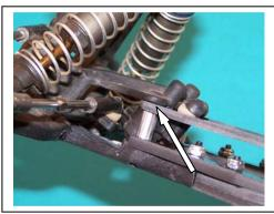
C5) Hold the front end on the truck and turn it over. Install the two flat head screws from Inst. #5. Finger tight for now.
