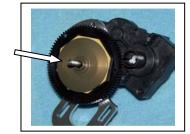
A27) Install the spring (AE9605) on the shaft so it goes around the slipper plate's hub, then place the black retainer over the spring, flat side up. Install the 5-40 nut (XF6074) to hold it all together, tightening until there is one thread of the shaft showing. Final adjustment later.
