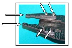
B4) Take the nose piece (XF1002) out of Bag B and check it for flashing, especially at the rear and on top of the post. We need good snug fit with the chassis and especially where the top deck fits on the post.
