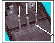
F4) Insert your antenna tube into the CF antenna mount (XF9001). Imagine that – a CF antenna mount! Be sure the tube extends down from the mount so the tube clears the top deck. Since we went to 2.4 gig spectrum the dreaded glitch-monster has mostly been sleeping, but if the antenna contacts the CF, that can him wake up. Use two 4-40 X 1/2" cap head screws and locking nuts to hold the mount on the top deck.
