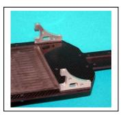
F3) Insert three 4-40 X 3/8" flat head screws up through the center of the chassis, place the last CF shim over the screws, and install the three 4-40 X 1" stand-offs (XF6801), If you use it, a drop of thread lock here.
