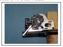
E2) Take the control arms (XF3011) from Bag E and remove the gurfelmurgles. A pair of pliers and a twisting motion seems to work best.
