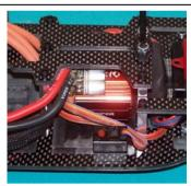
G7) Using servo tape, install the receiver in the right side of the center recess with the antenna wire forward. Run the wire up through the antenna tube, being sure to cage the glitch demon by keeping the antenna wire as far away from the CF as possible.
