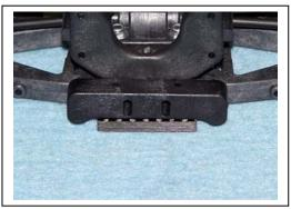
E14) In this photo we have inserted a pencil between the toe-in bar and the chassis to illustrate how the bar will slide up and down.
