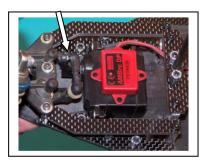
G5) Install the motor using the 3mm screws from your T 4.1. Chazz runs 17.5 blinky, so this is a 70-T spur and a 28-T pinion. To the moon!!!
