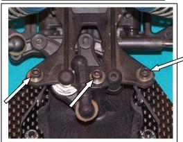
C7) Install the bumper with the screws from Inst #4.
