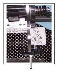
D9) We'll do the easy one first. Place a flat washer on a 4-40 X 3/8" cap head bolt, insert the bolt through the hole in the right front transmission tab, through the shim, and screw it finger tight into the cradle.
