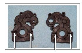
A14) Install a 3/16" X 3/8" rubber sealed bearing (XF6200) all the way into the top shaft boss in the left transmission case half (short arrow) and a 3/8" X 5/8" (XF6203) bearing in the boss for the differential. The Team pushes them in with the shank of an Allen driver or, better yet, with a socket. See Inst. A16.
