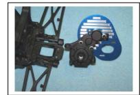
14) Remove the 5-40 nut which secures the slipper assembly, and pull off the nut, spring retainer, spring, outer slipper plate, outer slipper pad, spur gear, inner slipper pad, and inner slipper plate. The spur gear will not be used, so put it with the spares; save all other slipper parts for re-use.
