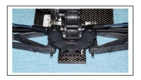
E13) Check the set-up sheet and tuning section to determine which toe-in bar (XF3211) you will use. Select the 3° or 4° toe-in bar and slide it onto the hinge pins. It will go above the chassis.
