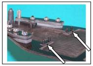
C2) Now install the two front deck supports, notch to the outside. A drop of thread lock now if you are using it. We must shim up the brackets because the X – 60CF chassis is 3mm while the SCX – 60CF chassis is 4mm.
