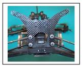
G3 Install the rear shocks to the front of the tower using all the parts saved from your T 4.1. Check the Set-Up sheet and Tuning guide; here we are using the 2 hole on the tower and 2 on the arms.
