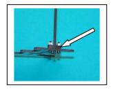
F5) Put two more 4-40 X 3/8" flat head screws up from the bottom of the chassis and install the two 4-40 X 7/8" stand-offs (XF6802) for the battery strap. A drop of thread lock here if you use it.
