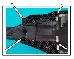
C4) Put the front suspension in its place, just as in your T4.1. The rear of the AE top deck fits over the center post and the two side holes fit over the stand-offs and front decks. Notice that in the left photo the center post is not properly engaged with the AE top deck. This must be a good snug fit, and the two side holes must fit snugly over the front decks. (right photo)
