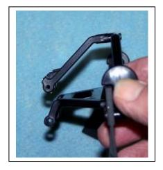
G12) Install the bumper on the bumper mount using four 4-40 X 5/8" cap head screws.
