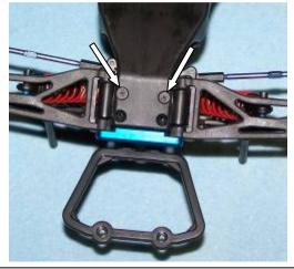
8) Remove the three flat-head screws and counter-sink washers which hold the top plate to the chassis. The entire front end and steering assembly should now come off the SC 10 as a unit. Save the assembly, screws &
