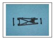
E3) The two arms are identical; when the arms are assembled to the truck, the shocks mount on the rear. However, we reverse the AE hub carriers, putting the right carrier (marked with an "R") on the left arm and the left carrier (marked with an "L") on the right arm. This makes the camber links line up better.
