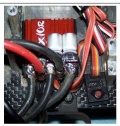
EL3) Mount the receiver on the left side of the chassis with double-sided tape behind the front top deck support. The antenna wire faces forward so the tube is close by. To prevent glitching, be certain the antenna wire touches only the tube.
