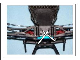
C4) Install the three bolts to hold the top deck to the front deck & standoffs and to the nose piece. Then put final torque on the two rear top deck bolts from C2.
