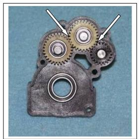
A18) Install the diff in the left transmission case bearing, ensuring it meshes properly with the idler gear. The head of the diff bolt should be up. Again, the transmission should be free and smooth.
