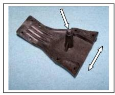
B5) Turn the chassis over and put the nose piece in place. Secure to the nose bridges with four 4-40 X 1/2" cap head screws (XF6002).
