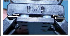
E16) Secure the toe-in bar and shims with two 4-40 X 1/2" flat head screws up from under the chassis. The screws go in the rearmost chassis holes, through the shim packs, and thread into the toe-in bar.
