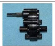
A21) Install the 4-40 X 3/8" cap head bolt (XF6001) in the lower corner of the trans case, just finger tight for now to hold things together.
