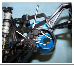
13) Remove the two button head screws from the top and two flat head screws from the bottom to take off the motor guard. Discard the motor guard, but hang onto the bolts.
