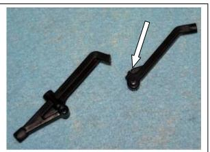
G11) Re-install the top bumper mounts just as they came off using the same bolts. You can throw away the front part which you cut off.
