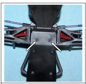
7) Still working beneath the chassis, remove the two flat head screws which hold the bulkhead to the chassis. Save these screws for reuse.
