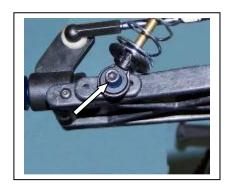
G5) We will install the nerf bars on the opposite side – right bar on the left side, left bar on the right. Use the 4-40 X 1/2" flat head screws and 4-40 locking nuts.
