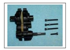
21) Remove the transmission components. The case will not be needed, but you will need the top shaft and spacer, two 3/16" X 3/8" bearings, idler gear with its two 3/16" X 3/8" bearings and shaft, and the differential assembly. The outdrive bearings will not be retained.
