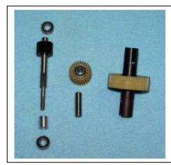
& two 3/16 X 3/8 bearings (XF6200). Replace parts as necessary.
