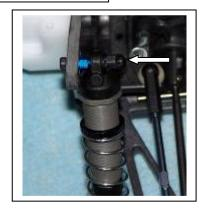
G4) Check the Set-Up Sheet and Tuning Section again, then install the shock bottom with the 4-40 cap head screw you took out. Don't forget the bushing! Here we are using the #2 hole.
