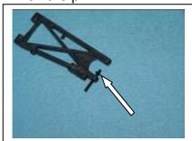
E5) Put the *right* hub carrier on the hinge pin.
