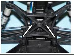
11) Remove the long bolt and captured nut that hold the two pieces of the bumper together. These will not be used.
