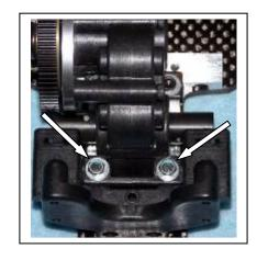
D11) Place a flat washer over a 4-40 X 3/8" screw, put the screw on your wrench, and fit it down between the transmission and the motor plate to secure the left front tab. Be sure the shim is in place (left photo). Now tighten both bolts and both nuts.
