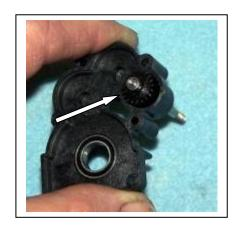
A16) Gather together the idler gear from the SC10 (AE9360) along with its 3/16" X 3/8" bearings (XF6202) and shaft (XF5201) along with the same parts from bag A so you have two gears, two shafts, and four bearings. Install a bearing into each side of both idler gears. Team drivers do it by pushing on the outer race with a socket.
