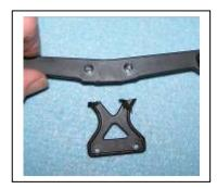
G7) Use the two 3/8" spacers and two 4-40 X 3/4" cap head screws to install the body mount to the bumper mount. The body mount extends to the rear now.
