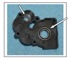
A15) Make sure the spacer (AE9602) is on the top shaft (AE9601) and slide the shaft with spacer through the bearing in the transmission case. If your top shaft is worn, you will want to try our one-piece steel top shaft (XF5210) made for us by M.I.P. No more spacer to lose and longer wearing too!
