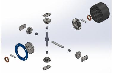
**Complete Assembly with Bearing/Ring Gear & Out Drive**
