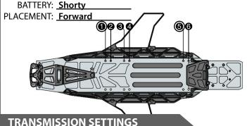
PINION: 22 tooth SPUR GEAR: 78 tooth DIFF. OIL: \_\_\_
