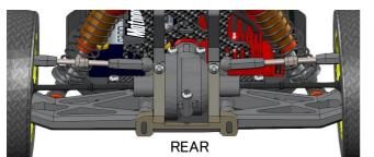
You have to install the differential case with reverse the left and right. (both front and rear)
