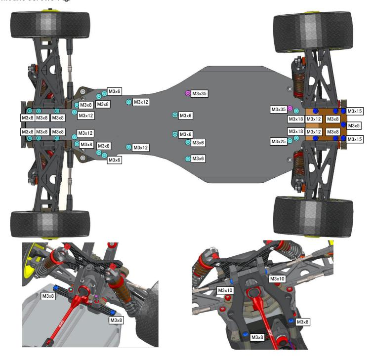
Cyan: Re-use flat head screw from DEX410 kit. Blue: Re-use button head screw from DEX410 kit. Mazenda: Included in DMX410 conversion kit.
