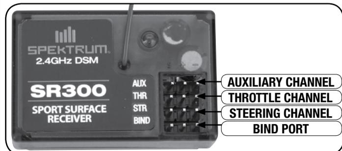
There is Bind, channel one, channel two and auxiliary slots.
