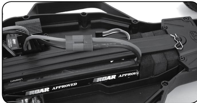
The battery hold-down has a flat side while the other side has strengthening ribs; the rib side should be face down to the battery. Insert on an angle into the rear support, and then down on the front pin and secure it with the previously removed clip.
