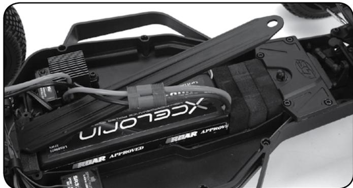
After you have inserted the fully charged battery pack, reinstall the battery hold-down strap.
