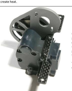
With the gearbox now fully tightened, add the slipper as it is supposed to be assembled on the RB5. Then add the rear Carbon Fibre brace. Make sure the countersunk holes are facing what will be the back of the car, as shown in the picture to the left (as we cannot see the countersinking from this view).
