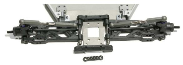
We have now the rear suspension fully attached to the car, it's time for the drivetrain.
