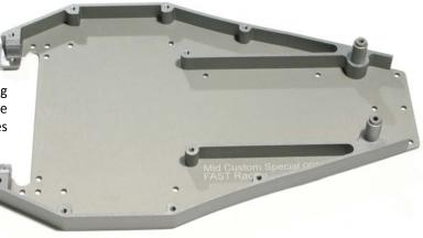
Next is to add the T-Plate holders, using 6 of the provided M3 x 6mm countersunk screws, as shown left.
