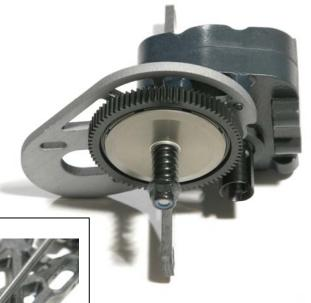
The gearbox should slot in nicely between the two suspension mounts, but the square section that slots inside the T-Plate can be a bit of a tight fit, so do not hesitate to push fairly hard. The gearbox is then secured on to the chassis by four M3 x 8mm countersunk screws, and the carbon fibre brace by two M3 x 10mm countersunk screws on to the chassis sides as shown.
