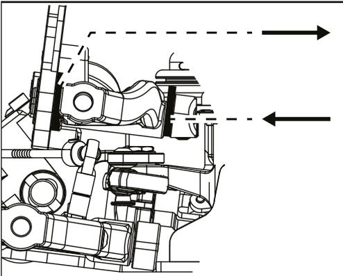
**Less caster (Clips back position)** – Gives more initial steering and less on-power (corner exit) steering – Useful to liven the car up on tight tracks.
