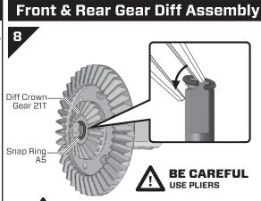
TEST FIT BEFORE SECURING THE SNAP RING
