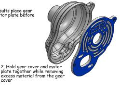
Cut the gear cover to alian with the edge of the motor plate
