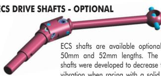
ECS shafts are available optionally in both 50mm and 52mm lengths. The ECS drive shafts were developed to decrease front wheel vibration when racing with a solid front axle, thus providing a much smoother and quieter ride and increased steering.
