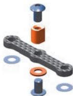
Smart chassis flex adjustment via graphite steering plate which can be mounted with an additional aluminum stand. Using only the graphite steering plate, chassis flex is medium; using the aluminum stand for reinforcement, the flex becomes stiffer. Stiffer flex results in more aggressive handling and increased steering.
