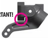
When adjusting steering on the radio, we recommend using full steering adjustment in order to get the best steering from the car. It is important to verify that the steering block does not touch the C-hub; that would lead to chassis tweak due to extra servo strain.
