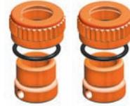
Very handy, easily externally adjustable body post from Swiss 7075 T6 aluminum. Allows for adjustment of body height by 3mm without needing to change the position on the body post.
