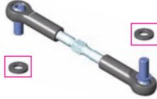
The angle of the ARS linkage – which is made by adding/removing shims on the steering block and ARS post mount – changes the toe-in characteristics of the rear tires under rolling effect; when the car is pressed the toe-in can either increase or decrease.
