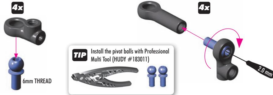
**TIP** Install the pivot balls with Professional Multi Tool (HUDY #183011)
