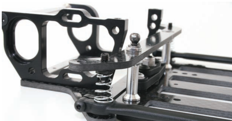
Below: Springs control the roll of the rear pod
