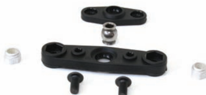
Above: This is the ball joint that has basically replaced the T-bar of the original
