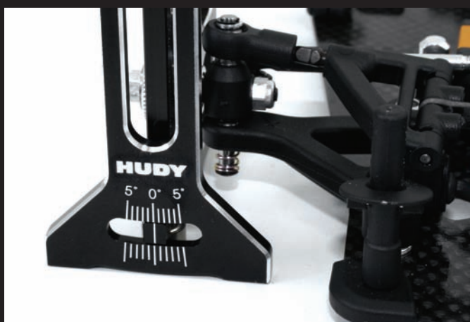
Above: Camber adjustment can be accurately measured
