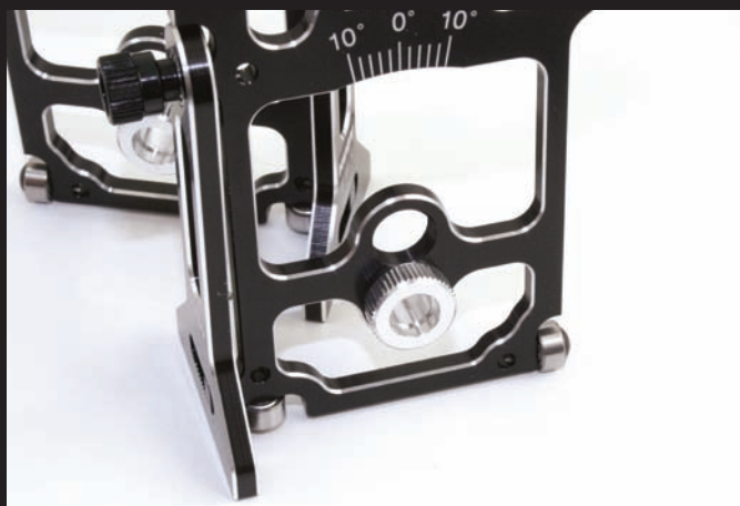
Above: Bearing insert, upper for tenth and lower for twelfth
