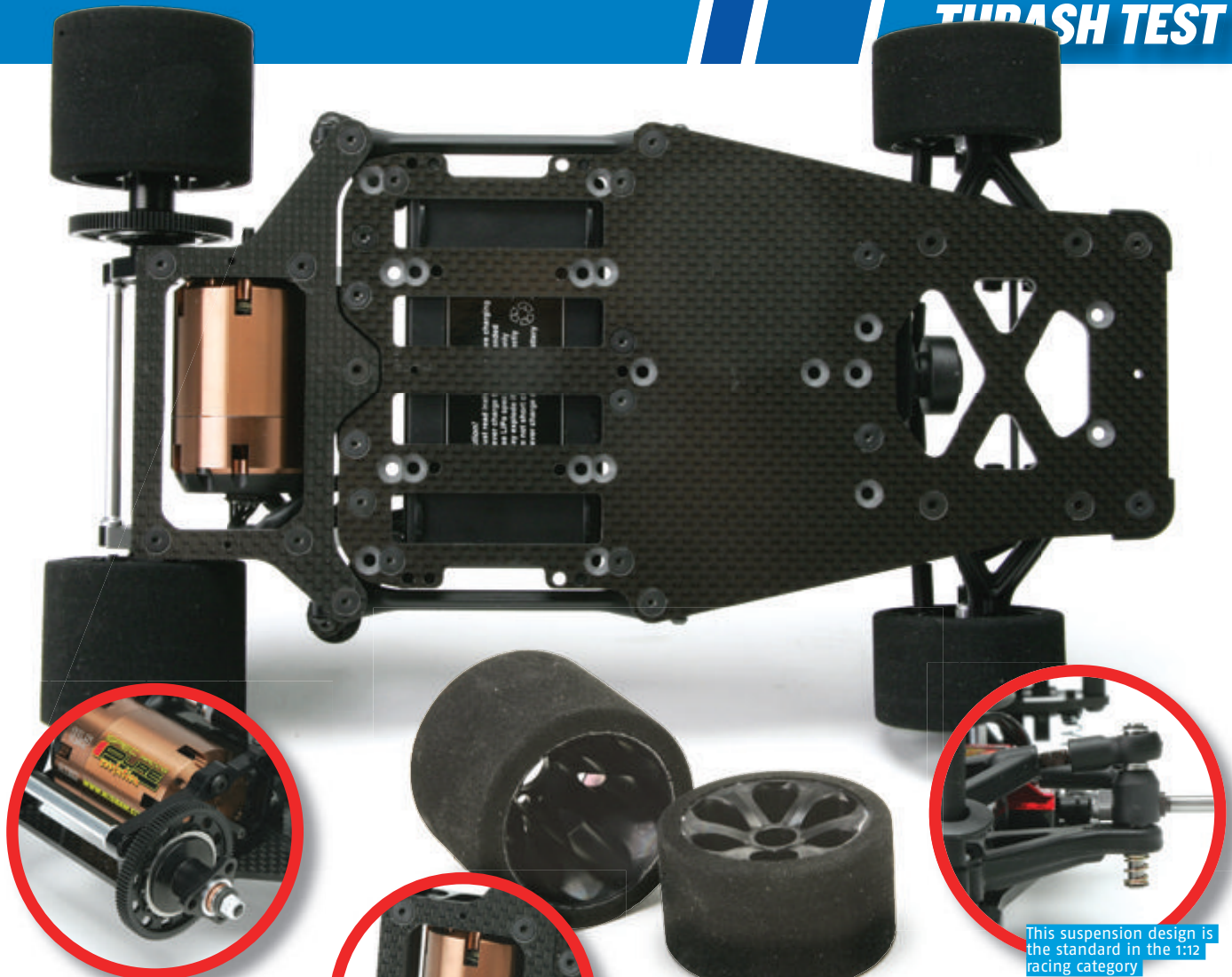
Ball differential uses a proper thrust bearing for ultra-smooth operation and longevity
