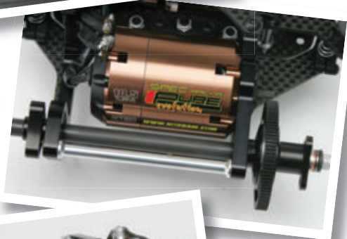
A Nosram 10.5T motor was a breeze to install into the Xray XII Link with lots of space around the pod area
