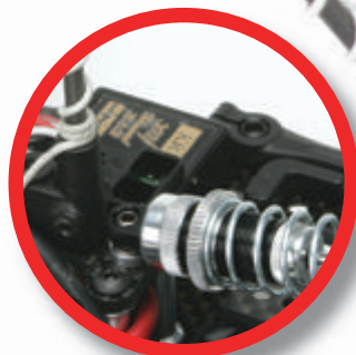
Threaded bodied, oil-filled centre shock is of the traditional design
