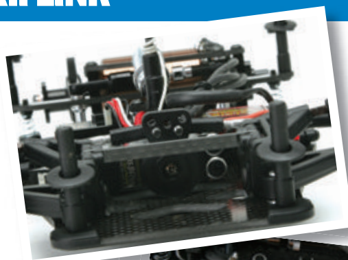
Front suspension is connected by a carbon fibre strut although an Aluminium Active Brace Set is available as an option
