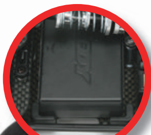
Ready LiPo is securely located in the chassis with its shaped case and Xray's moulded retainers
