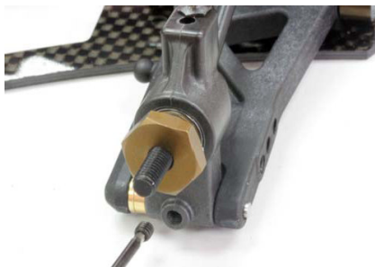
Step 45 - Secure the 2.5mm suspension pin with a set screw.
