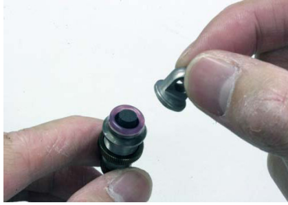
Step 60 - Put on damper diaphragm, optional pressure sponge and top metal ball link. Note. Pressure sponge is optional and not included.
