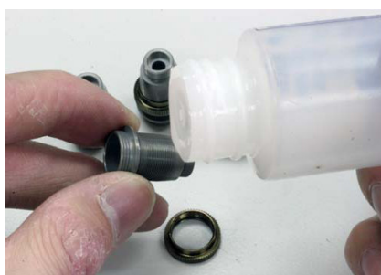
Step 56 - Shock Installation: Lubricate shock body with damper and screw on adjuster.
