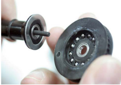
Step 16 - Install diff. ring with diff. grease to the long diff. hub; install it to the centre of diff. pulley; make sure the side of pulley is correct.
