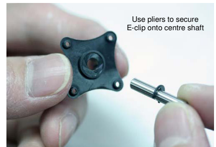
Step 24 - Insert centre shaft into centre pulley.
