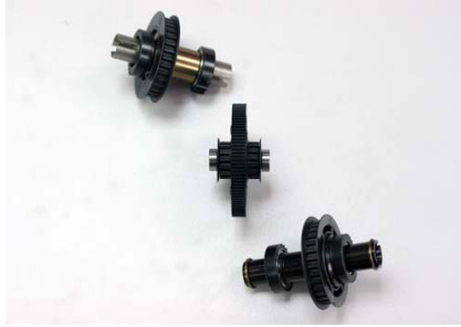
Step 29 - Install tension adjusters onto bearings of both front one-way and rear diff.
