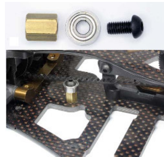
Step 66 - Place one 3x8 bearing on top of tensioner post and secure the assembly by screws on top and bottom.
