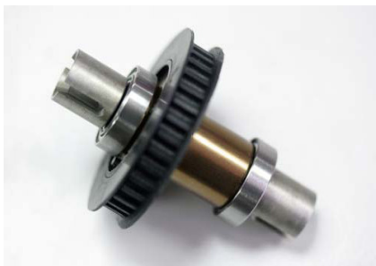
Step 22 - Fit front one-way shafts and 1510 bearings, the front one-way is now assembled.
