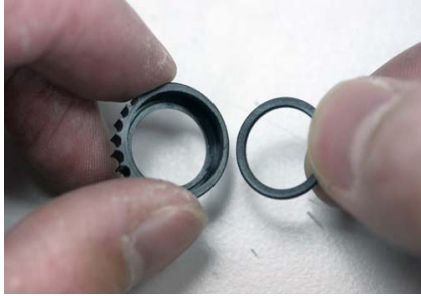
Step 28 - Place a tension adjustment spacer in each tension adjuster for front one-way assembly.
