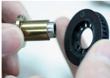
Step 20 - Install front one-way to diff. pulley. Note direction.
