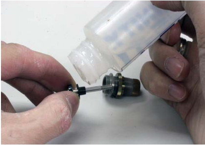
Step 58 - Assemble shock shaft and spacer; Add damper oil for lubrication. Insert shaft into damper case and tighten damper bottom.
