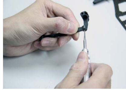
Step 5 - Pre-tap all screw holes of all plastic (use M3 tapping tool if available).
