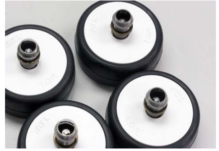
Step 59 - Add damper oil into shocks and allow them to settle to remove air bubbles.
