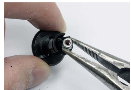
Step 12 - Place the diff. nut inside the diff. nut slot at the centre of the short diff. hub. Use small Allen wrench to hold in place.
