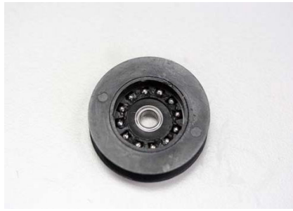
Step 14 - Apply diff. grease and install diff. balls; install diff. pulley adaptor with bearing from step 13.
