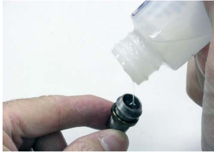
Step 59 - Add damper oil into shocks and allow them to settle to remove air bubbles.
