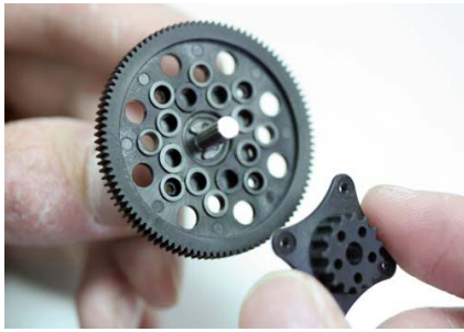
Step 25 - Insert spur onto centre shaft and then fit the second centre pulley.
