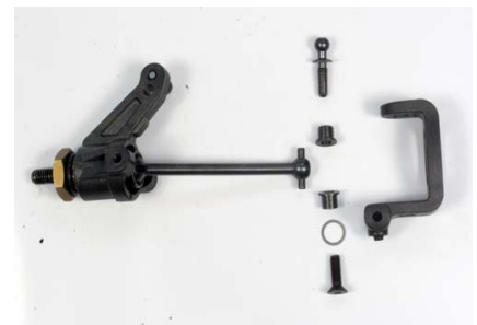
Step 46 - Assemble steering hub carrier. You can fit the wheel nut until later.
