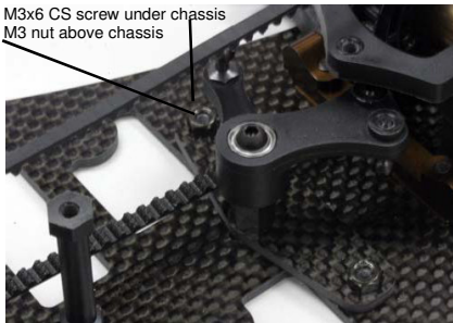
Step 39 - Install the steering assembly onto the main chassis deck just behind the front suspension assembly. Check set-up sheet..
