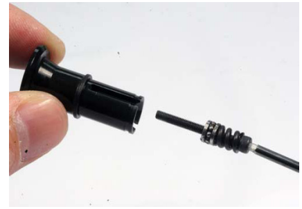
Step 15 - Apply thrust grease, install the thrust bearing and spring through the diff. screw and through the centre of long hub.
