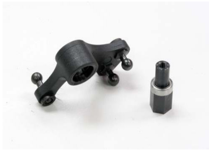
Step 36 - Screw ball studs (short) into steering crank - use 5.0mm hex socket driver
