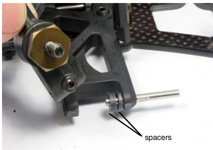
Step 44 - Install left rear knuckle; make a symmetric installation on right hand side.
