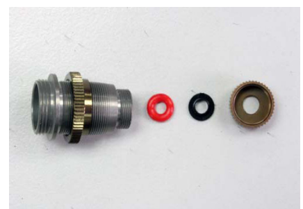
Step 57 - insert o-ring then spacer into damper then screw on bottom cap.
