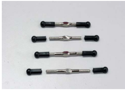
Step 48 - Assemble 4, 34mm camber link tie rods and a further 2, 45mm tie rods for steering links.
