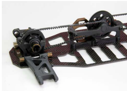
Step 31 - Insert front one-way into front drive belt and rear diff. into rear drive belt and insert centre pulley assemblies onto main deck. Ensure tension adjuster is located into the bulkhead and belt tension is suitable. The belt drive assembly is now complete.
