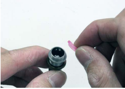
Step 60 - Put on damper diaphragm, optional pressure sponge and top metal ball link. Note. Pressure sponge is optional and not included.
