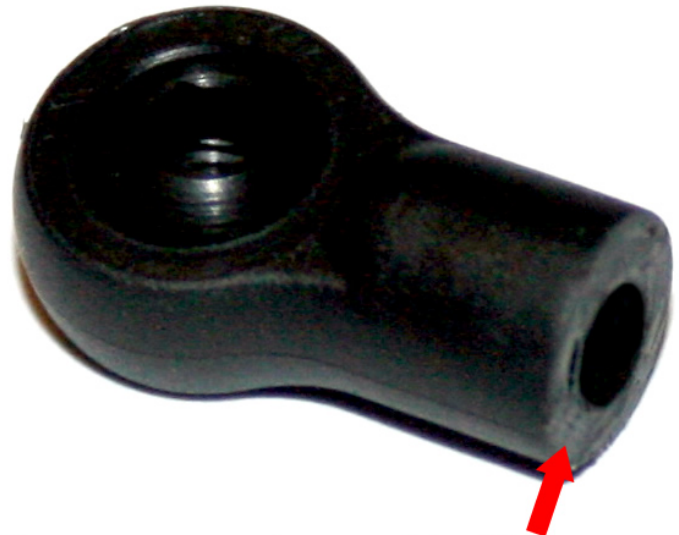
Ballcup cut on the molded line
