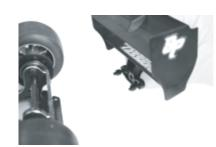
2 Slide the rear wing mounting screws through the rear wing mount and secure with (2) M3 lock nuts
