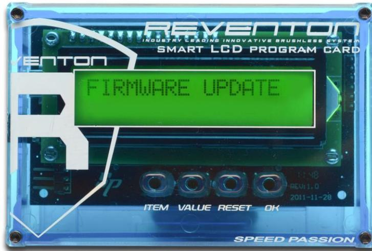
4. The program card will be display “FIRMWARE UPDATE “. Release the “RESET” button and launch the “Speed Passion Reventon PC Interface” program.
