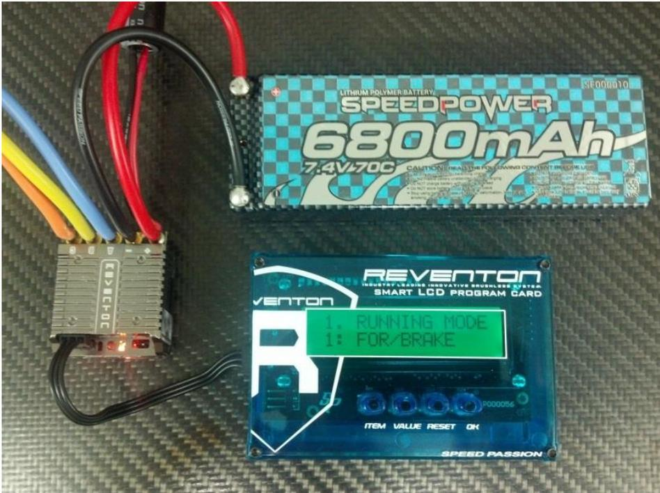
1. Disconnect the battery from ESC.
