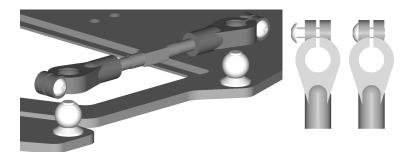
Next, attach only one of the link assemblies to the suspension balls on the chassis. Insert the 2-56 x 1/4" button head screw (smr2060) into the clearance (larger) hole, and screw in until it just bottoms on the captured link ends. It is extremely important that the captured link ends do not bind on the 1/4" x 4-40 suspension balls.
