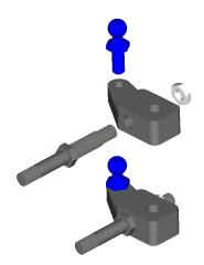
Install the axle assembly (x2) into the steering block as shown. The axles screw in with a left hand thread into the steering block. The nut on the back side has a standard right hand thread.
