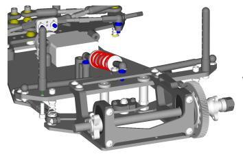
Locate the body posts and attach to the tweak plate with  $4-40 \times 3/8$ " long socket head cap screws (x2).
