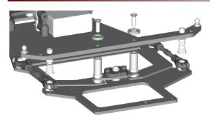
With the tweak spring holders adjusted all the way up, install onto the chassis using 4-40 x 3/8" flat head screws (x2) through the countersunk washers (x2), into the stand-offs.
