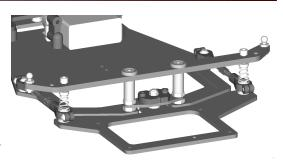
After locating 1 aluminum ball stud, the shock/antenna mount, and 4-40 x 3/8" screws (x2), install the shock mount in the orientation as shown.
