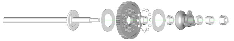
From left to right shown above is; the rear axle, differential ring, 88 tooth spur gear, 3/8" x 1/4" unflanged bearing, 1/8" differential balls (x12), differential ring, 3/8" x 1/4" flanged bearing, thrust cone, nylon differential nut.
