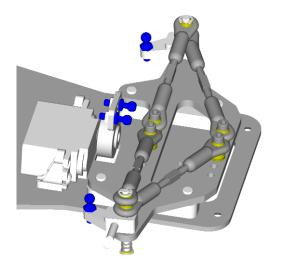
After carefully marking the center of the servo mounting holes, place the assembled servo back on the chassis to make sure the marked holes appear where they should be.
