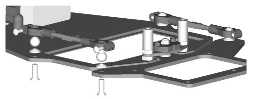
Next, place two 4-40 x 3/8" flat head screws through the chassis and lower pod plate on the opposite side. From the top of the chassis, place one low roll center cone on each of the screws, followed finally by a 4-40 threaded ball screwed down tight. Next attach the second link to the opposite side using the same method as before.
