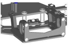
Next, attach the rear carbon fiber pod plate using 4-40 x 1/4" button head screws (x4), again being sure not to over-tighten.
