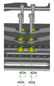
Using the  $4-40 \times 5/8$ " socket head cap screws (x4), brass cone washers (x4) and large 4-40 lock-nuts (x4), attach the links to the lower arm. Slide the screws through the captured ball ends then through the cone washers, then thread them into the holes closest to the center of the chassis. Keeping a hex driver in the screw, use a nut driver to install the 4-40 nuts from below the chassis. The screws should be held snug to the carbon lower arm when tightening the nuts.
