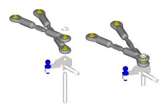
Locating the kingpins (x2), and the previously assembled front links and steering blocks, along with 1/8" E-clips, assemble as follows; Install the kingpin into the steering block to about the middle of the kingpin. Next, slid on the longer link (front) first followed by the shorter link (rear). Install the E-clip onto the top of the king pin. Now slide the steering block to the top of the kingpin, taking up the slack at the top of the kingpin.
