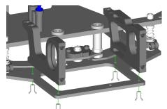
Locate the bulkhead plates for the rear pod and 4-40 x 1/4" flathead screws (x4), and attach to the lower pod plate as shown, being sure not to over-tighten.
