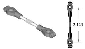
Assemble the side links from the Link Set (smr1264), screw onto each end of the turnbuckles one of the captured link ends (smr1265-s). Space the plastic captured link ends equally 2-1/8" apart from center to center. This will get the link close, and will be fine-tuned later.
