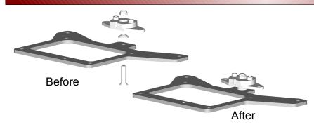
Attach rear pod plate to the center pivot using a 4-40 x 1/2" flat head screw (smr2014). Use a low roll center cone (SMR5008) on top of the lower pod plate, screwing through the 1/4" x 4-40 threaded suspension ball in the center pivot. Secure using a 4-40 mini-locknut (SMR2080) as a jam nut.
