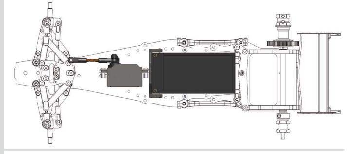
Detail view forward battery and servo configuration
