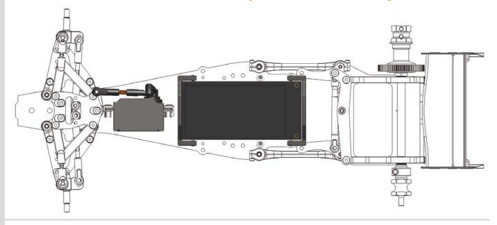
Detail view forward servo and rearward battery configuration
