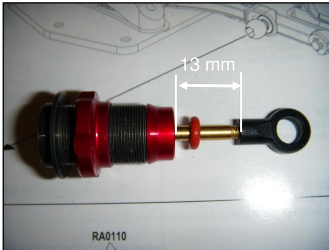
*The Shock Absorbers assy is a pure pleasure. Make sure to always lubricate all the element with the oil you will use, especially on the bladder which will first be installed inside the upper cap before being screwed onto the body.*
