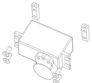
Use the 4 x HW008 M3x8 countersunk screw to fix the FX022 servo mount.
