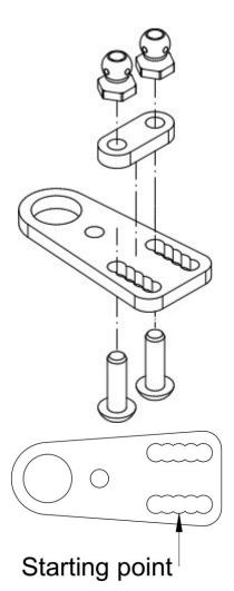
Assembly the steering linkage as shown. Take some care when insert the bearings in the carbon fibre.
