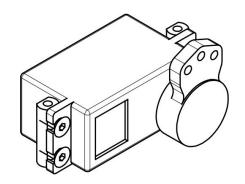
Assembled group. Servo saver should be vertical when servo is neutral.
