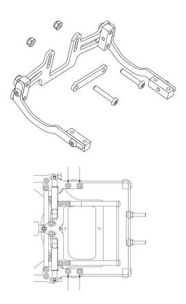
Use 4 x HW003 M3x8 button screw and assembly the M20-6 wing holder to the shoulders
