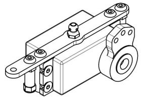
Using 2 x HW008 M3x6 Button, fix the servo group to the M33-10 servo holder
