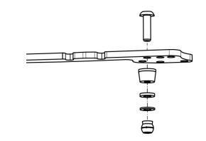
Insert the G56042A spacer between the carbon side wing and the link sphere.
