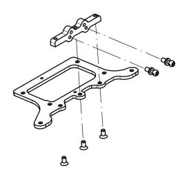
Using 3 x HW012 M3x6 countersunk screw fix the V-link F2 to the M33-4 motor pod.
