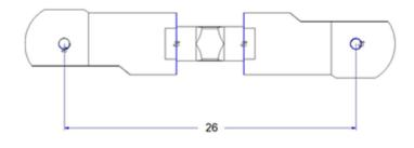
Keep this dimensions. Fix the link over the V-link F2
