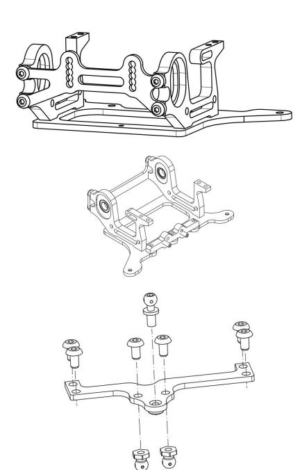
Fix the M33-6 wing stay to the group using 4 x HW008 M3x6 button screw.
