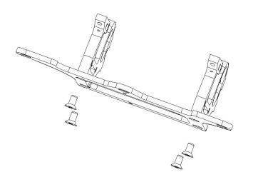
Using 4 x HW012 countersunk screws, fix the motor holder to the motor pod.
