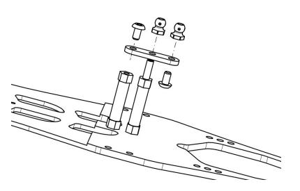
Fix the M33-7 mini shock holder using 1 x HW003 M3x8 button screw, 1 x HW034 M3x15 grub screw and one FUFX48 as show.
