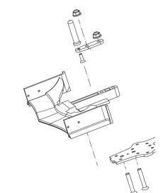
Now you can couple the motor pod to the chassis group. Use the M33-5 shock holder, using 4 by HW008 3x6 button screw.
