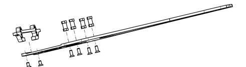
Assembly 4 x FX0052 12mm post with 4 x HW007 M3x8 countersunk screw
