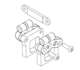
Secure the G56-030 upper arm mount to the M20-16 using 2 HW004 M3x10mm Hex button screw
