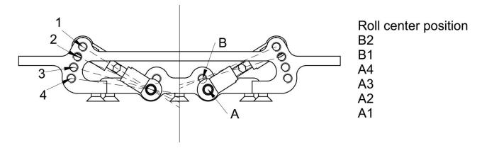
V-Link suspension has the unique ability to alter the roll centre position.
