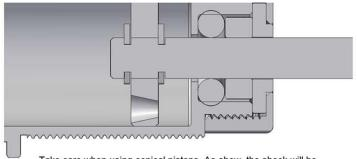
Take care when using conical pistons. As show, the shock will be harder in compression and softer in extension
