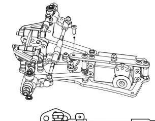
Use one HW003 M3x8 button screw to fix the M33-10 to the steering post.
