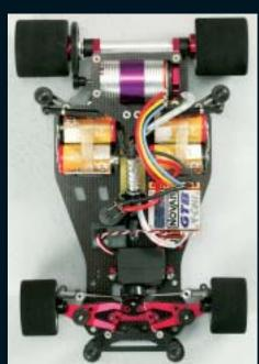
The SP12X offers a lightweight 2.4mm wovengraphite chassis. In the U.S. spec kit there are minimal cutouts, making the car ultra stiff on high-traction applications
