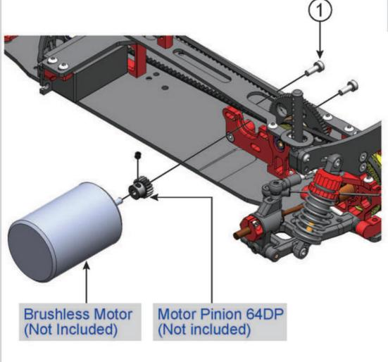
Gear mesh should have a minimal amount of play between spur and pinion.
