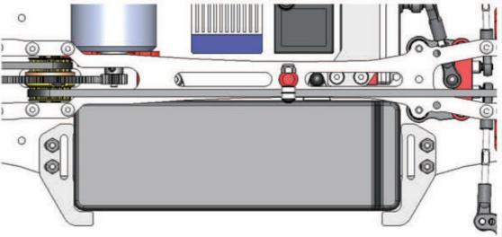
Battery location can be adjusted by moving the battery holder.
