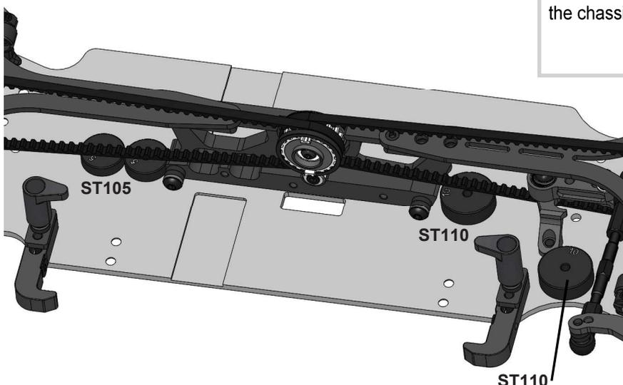
The engraved sides of **ST110** and **ST105** are flat. The opposite sides are chamfered.
