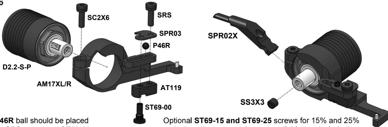
Note: **P46R** ball should be placed between **SRS** screw and **ST69-00** screw.
