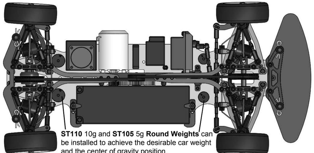
**ST110 10g and ST105 5g Round Weights** can be installed to achieve the desirable car weight and the center of gravity position.
