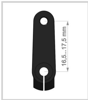
**Note:** Recommended length of the servo horn at the long servo link layout is 16,5-17,5 mm.
