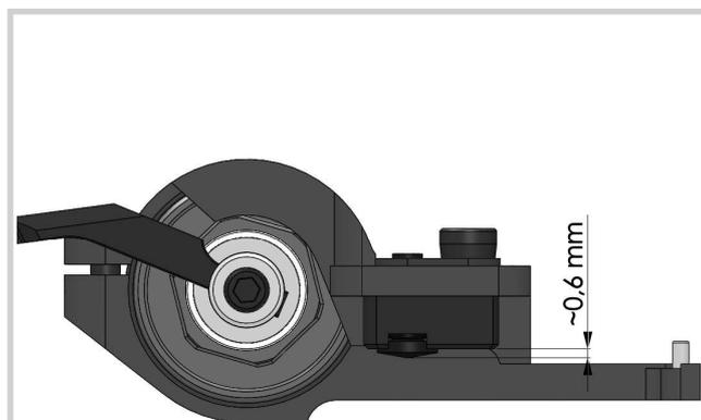
**Note:** Initial position of **ST69-0** Screw is ~0,6mm.
