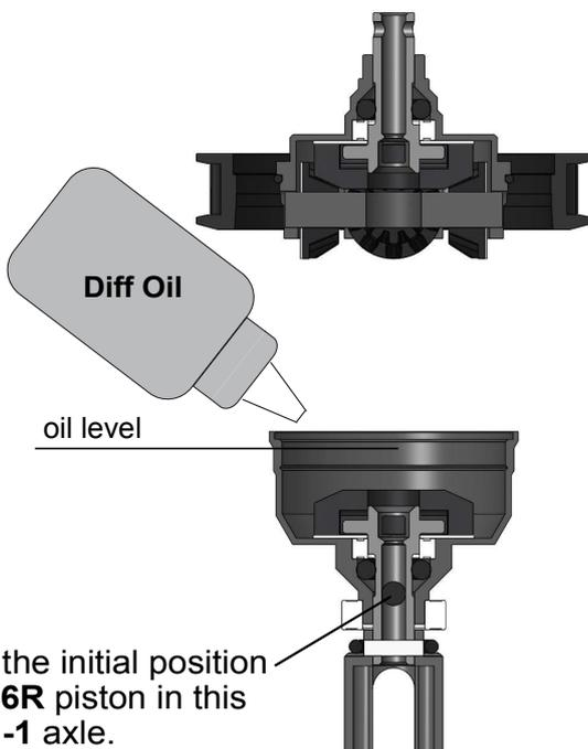
Note the initial position of **P46R** piston in this **ST31-1** axle.
