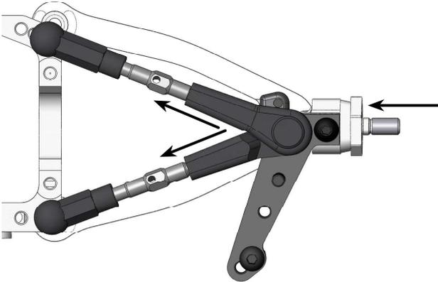
**Caster adjustment rule:** Simultaneous front upper rod 0.5mm elongation and rear upper rod 0.5mm shortening adds 2.5° of caster at constant camber.
