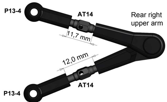
**Notes:** The given rods and arms sizes are approximately for 4° front caster and 0° rear caster, 2° both front and rear cambers, 3,0° rear toe-in and 1° front toe out angles. Use a setup station or angles gauge for further precise suspension geometry setting. See our recommendations on page #23 for quick and easy suspension geometry change.
