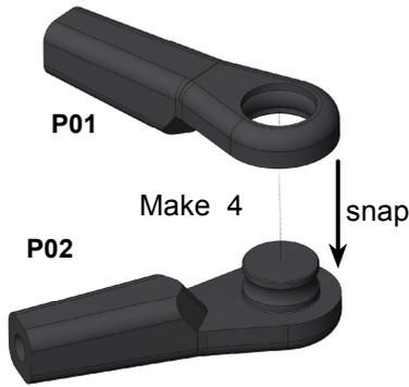
Servo rod for long servo link layout
