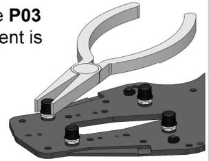
**Note:** Use other combinations of **SH0.5**, **SH1.0** and **SH1.75** spacers under appropriate **AT21ST-A** balls to adjust your car set-up.
