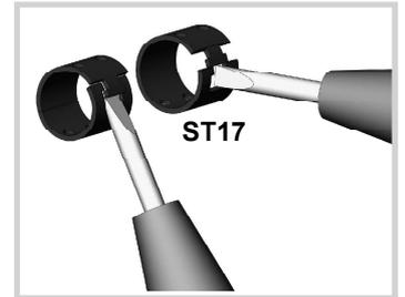
1. Insert a 2.5mm flat screwdriver tip into **ST17** Universal Ring slot, bend of the lug and turn screwdriver through 90 deg.
