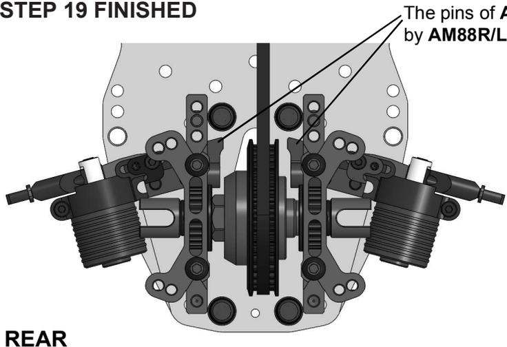
The pins of **AM17** should be covered by **AM88R/L** Shock Holders.
