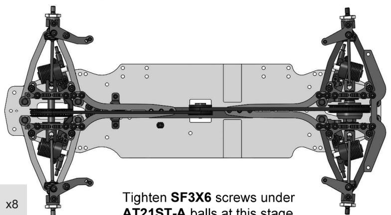
Tighten SF3X6 screws under AT21ST-A balls at this stage.
