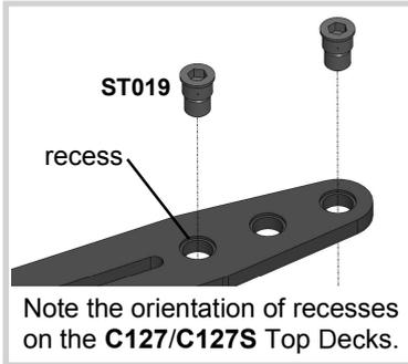
Note the orientation of recesses on the C127/C127S Top Decks.
