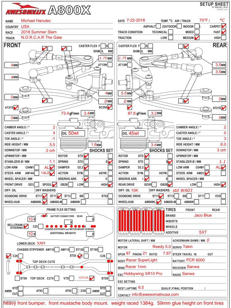
same setup as Mile High. Similar to Gee's setup but with short alloy arms so reduced front A-gap by 0.6mm.
