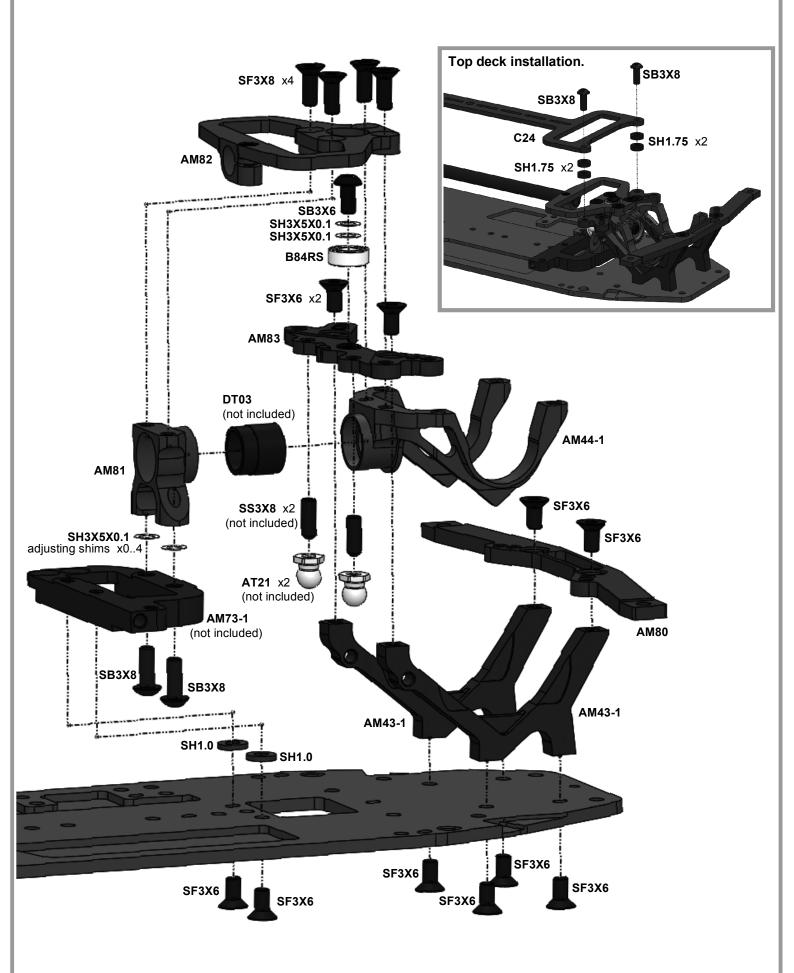
Note: 1. AM73-1, DT03, AT21, SS3X8 are the parts of the car kit.
