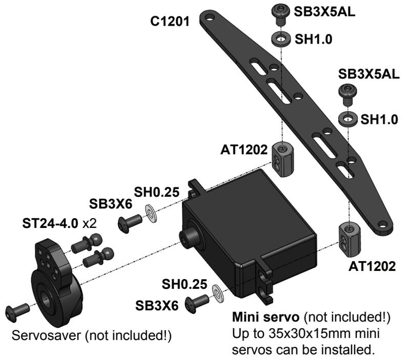
**Note:** ST24-4.0 are 4.0mm ball studs. ST24-4.0 fit P1213 4.0mm ball cups.
