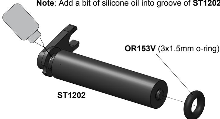
**Note:** Lubricate **OR153V** via silicone oil. Stretch **OR153V** via fingers and put it on **ST1202** (to avoid the damage of o-ring please don't use a sharp edged tool for this!).
