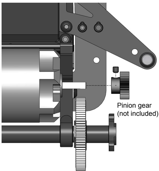
**Note:** The sum of the 64P spur+pinion teeth should be within 112-120 range for short wheel base and within 112-125 range for +1mm longer wheel base.
