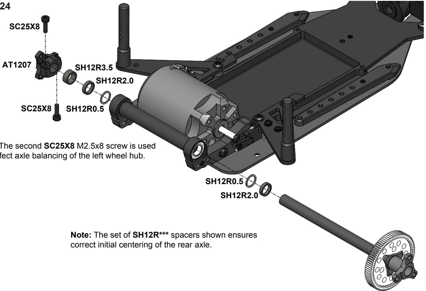
**Note:** The second **SC25X8** M2.5x8 screw is used for perfect axle balancing of the left wheel hub.
