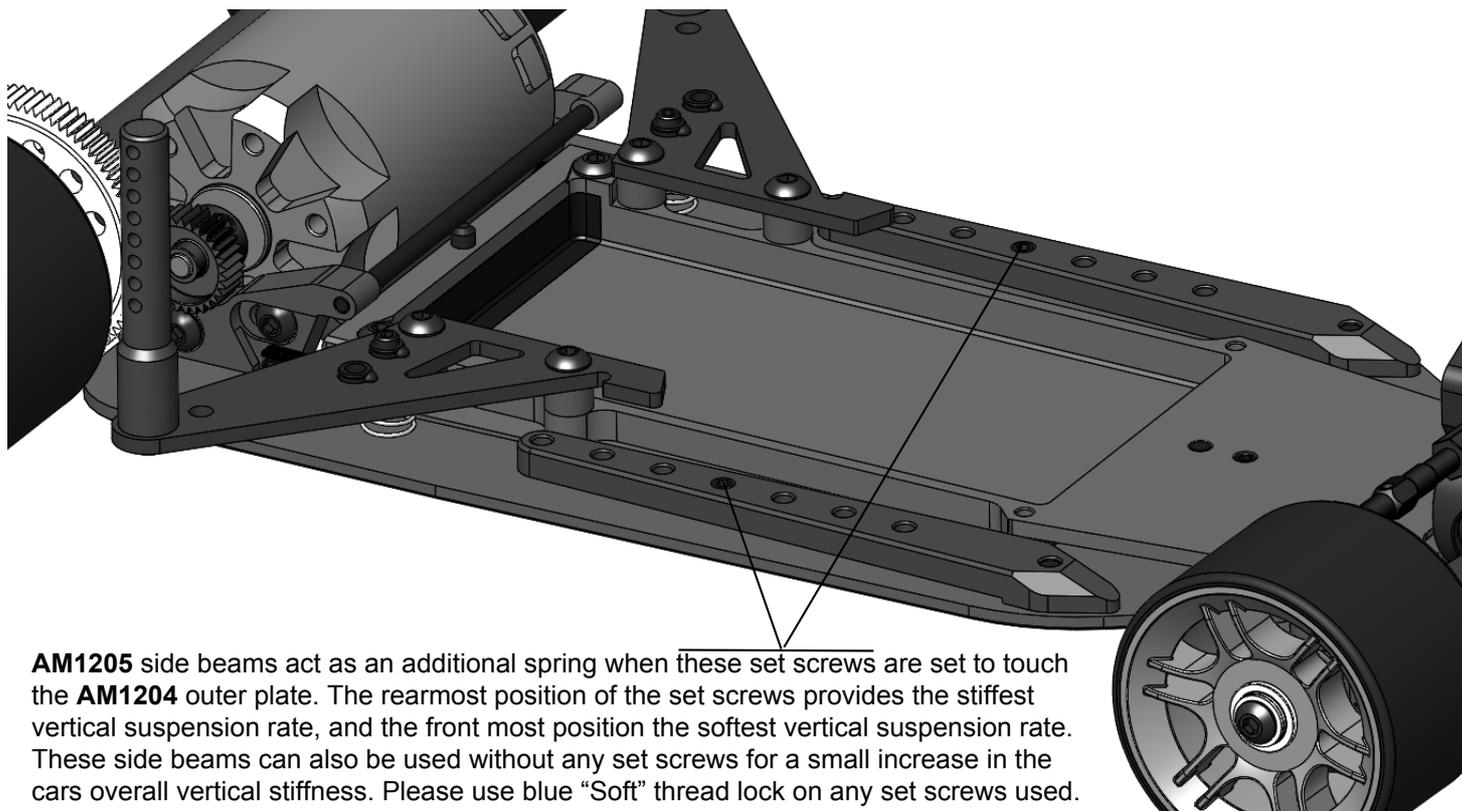
**AM1205** side beams act as an additional spring when these set screws are set to touch the **AM1204** outer plate. The rearmost position of the set screws provides the stiffest vertical suspension rate, and the front most position the softest vertical suspension rate. These side beams can also be used without any set screws for a small increase in the cars overall vertical stiffness. Please use blue "Soft" thread lock on any set screws used.
