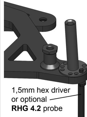
Alignment of the appropriate holes of **ST1208** and **C1205** for camber settings.
