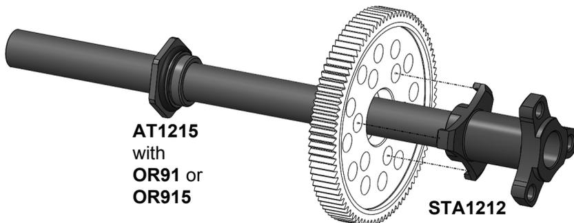
**Note:** Tighten AT1215 nut via 12mm wrench. Please don't overtighten AT1215 nut!
