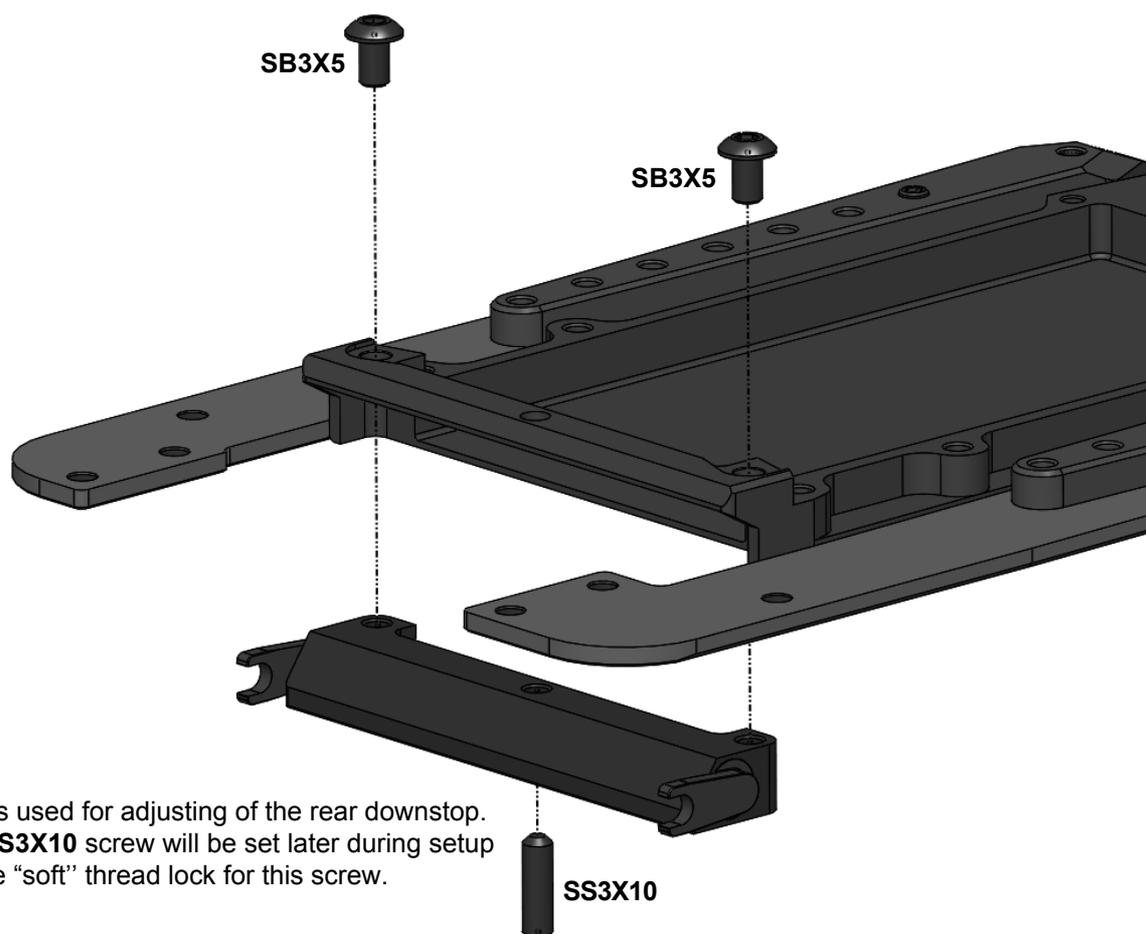
**Note:** **SS3X10** set screw is used for adjusting of the rear downstop. An exact position of this **SS3X10** screw will be set later during setup of the car. Please use blue "soft" thread lock for this screw.
