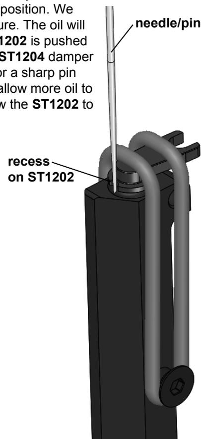
**Note:** It is very important to assemble the damper without any air inside! The silicone oil has to occupy the gap between the damper's rotor and case fully. It can take some practice.
