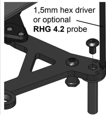
The tip of 1,5mm hex driver or optional **RHG 4.2** probe is used for alignment of the appropriate holes of **ST1208** and **C1205**.
