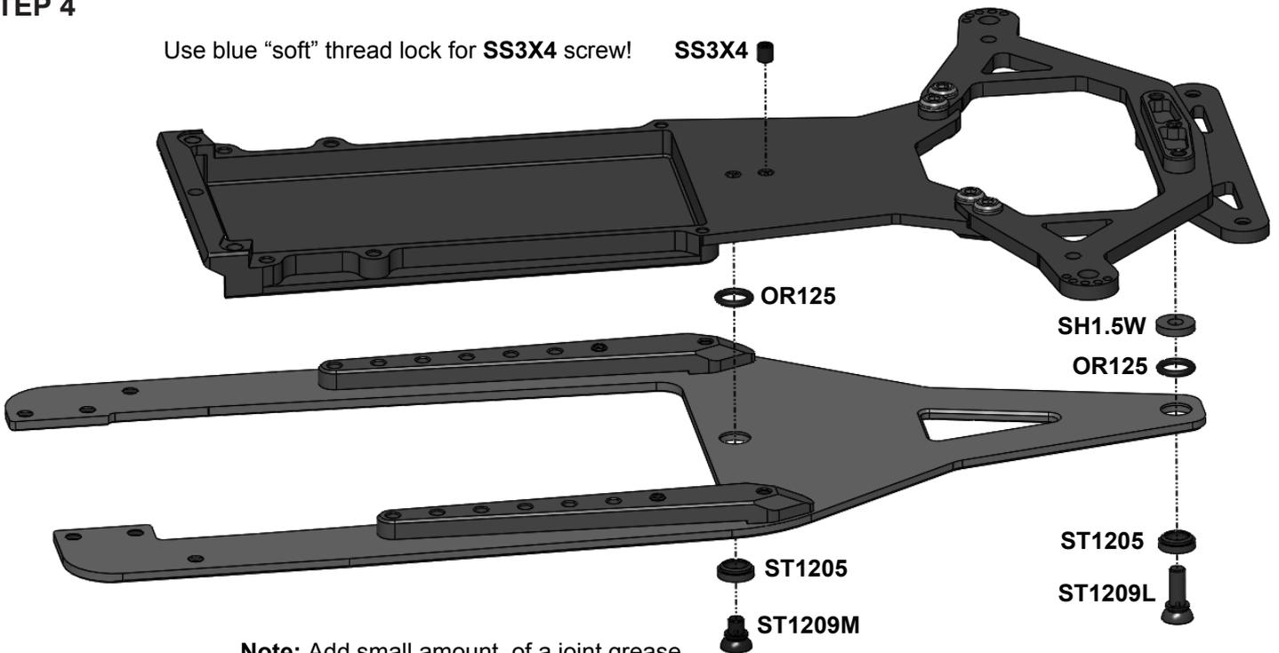
**Note:** Add small amount of a joint grease between **ST1205** and **ST1209M/L**.
