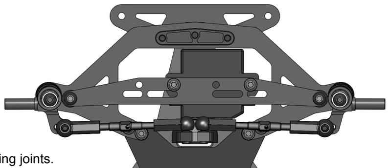
**Note:** P1213 4.0mm ball cups are used for the inner steering joints.
