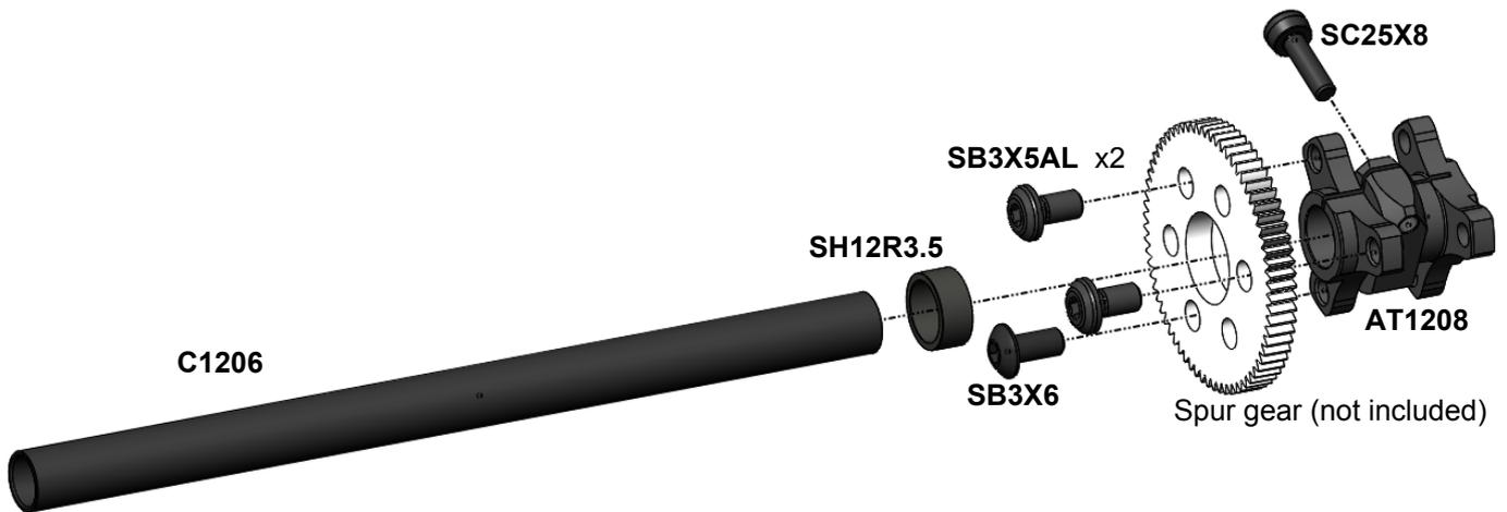
**Note:** Optional **ST1212** steel axle can be used instead of **C1206** carbon axle.
