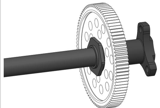
**Note:** The sum of the 64P spur+pinion teeth should be within 112-120 range for short wheel base and within 112-125 range for +1mm longer wheel base.
