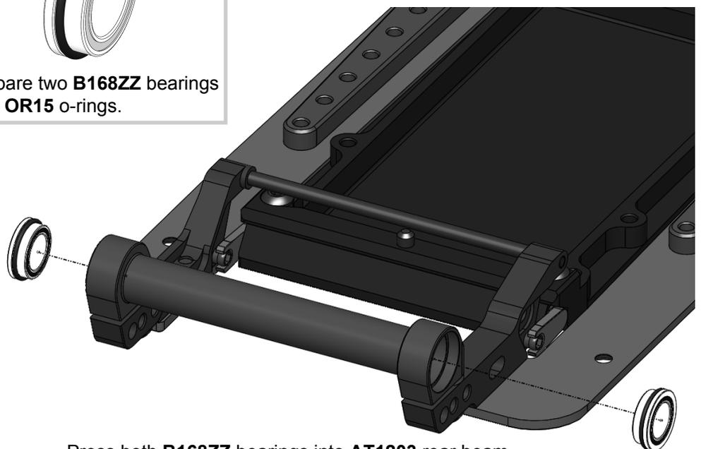
Press both **B168ZZ** bearings into **AT1203** rear beam.
