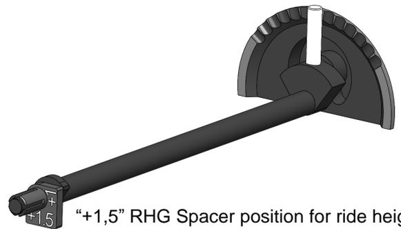
"+1,5" RHG Spacer position for ride height measuring within 4.5 - 5.7mm range.
