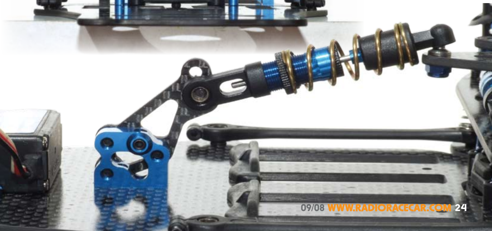
Below: The radical new damper design; note the piston rod at each end. Adjustable angle as well
