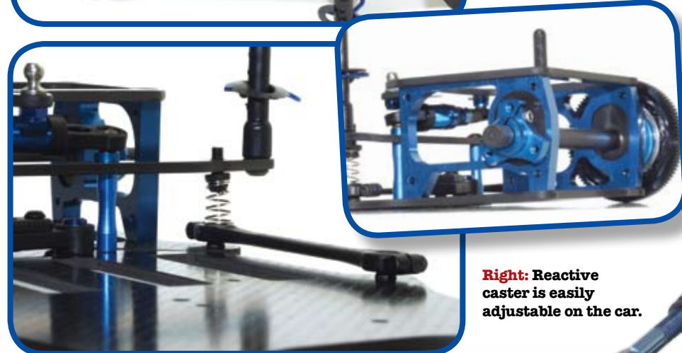
Above: The rear side link and spring, note that the link ball joints are adjustable to get a snug fit
