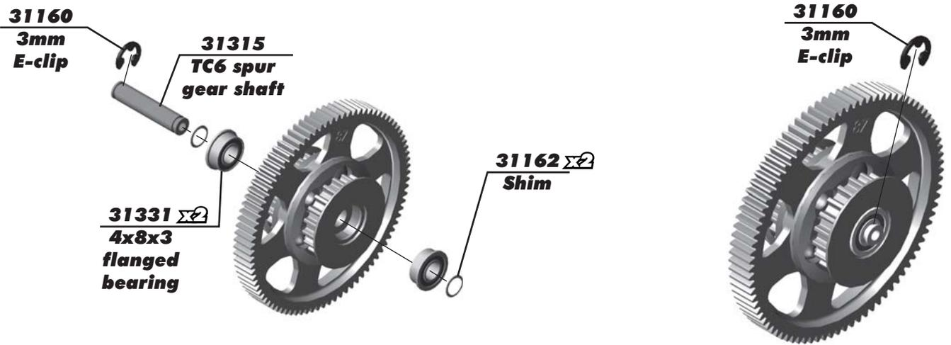
**:: Spur Gear Hub / Belts Install - Bag F - Step 1**
