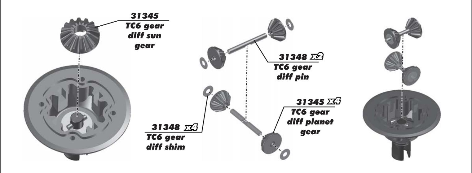
**:: Rear Gear Differential Build - Bag B-BB - Step 3**
