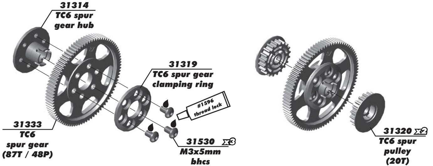
**:: Spur Gear Shaft Build - Bag F - Step 2**
