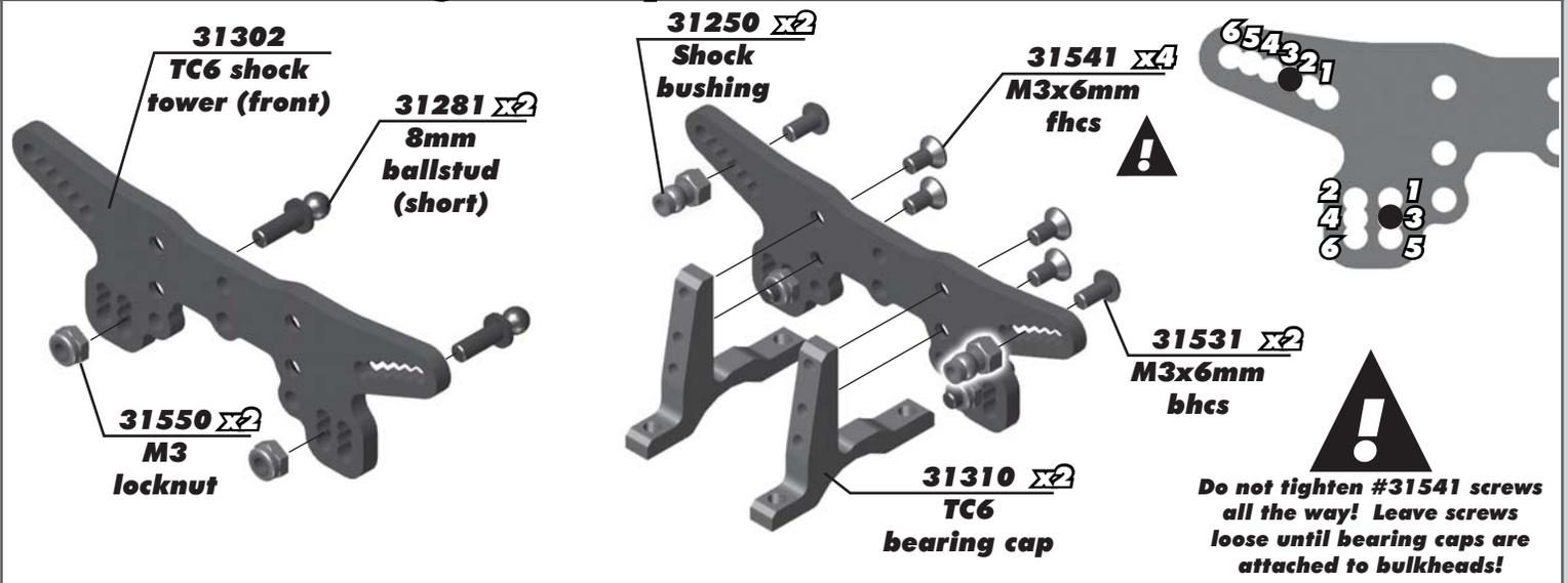
**:: Shock Tower Build - Bag D-DD - Step 2**
