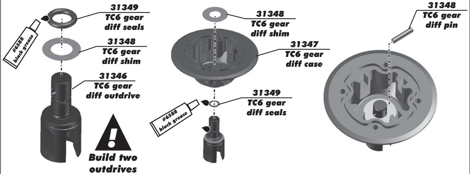
**:: Rear Gear Differential Build - Bag B-BB - Step 2**
