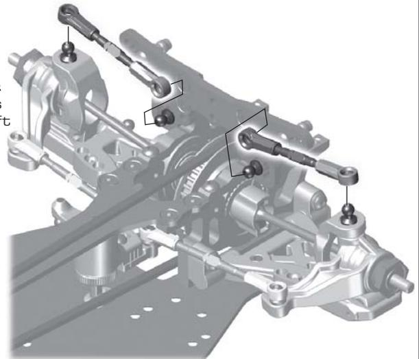
**:: Steering Block Build / Install - Bag G - Step 8**
