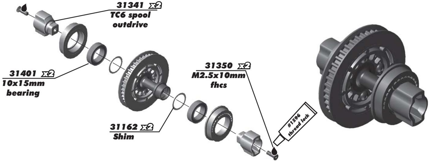
**:: Rear Gear Differential Build - Bag B-BB - Step 1**
