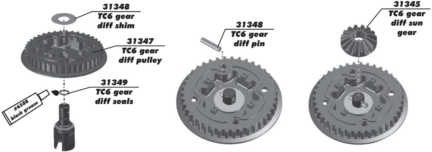
**:: Rear Gear Differential Build - Bag B-BB - Step 4**
