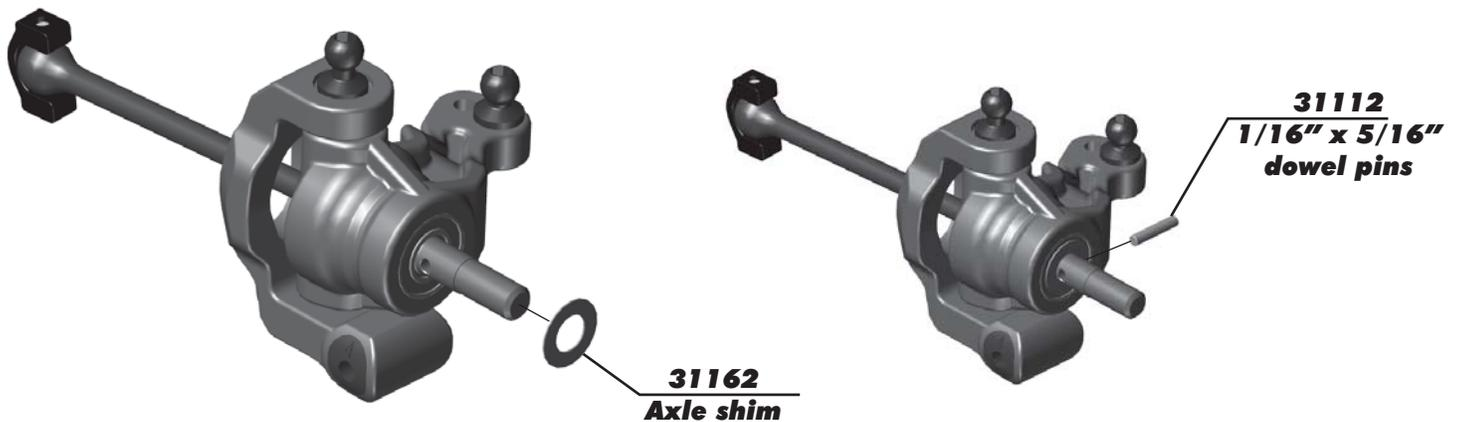
**:: Steering Block Build / Install - Bag G - Step 6**
