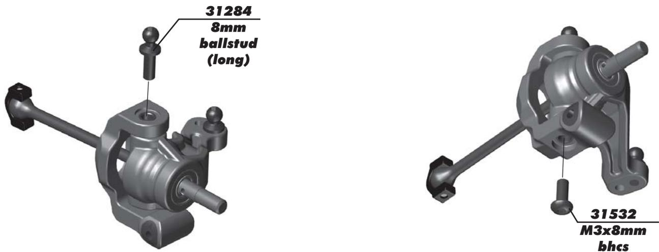
**:: Steering Block Build / Install - Bag G - Step 5**
