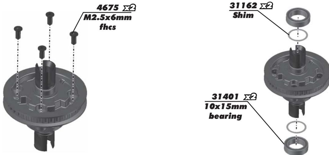
**:: Rear Gear Differential Build - Bag B-BB - Step 6**
