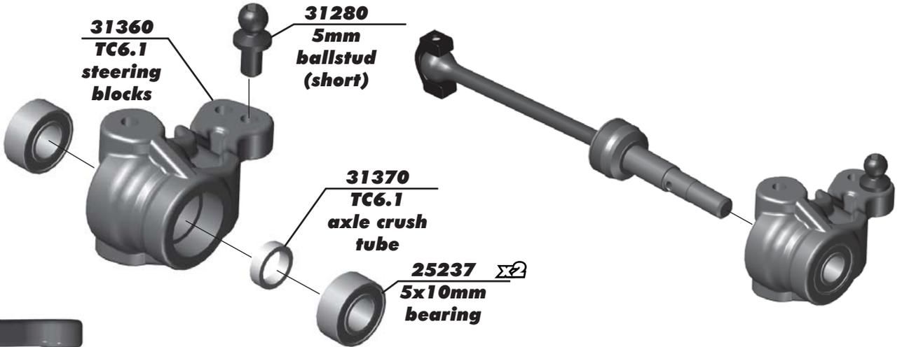
**:: Steering Block Build / Install - Bag G - Step 2**
