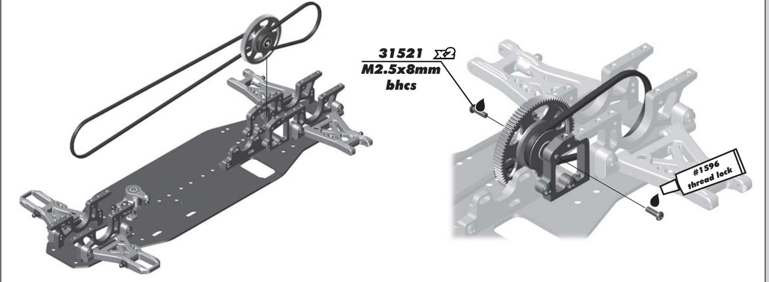
**:: Front Spool / Rear Gear Differential Install - Bag F - Step 1**
