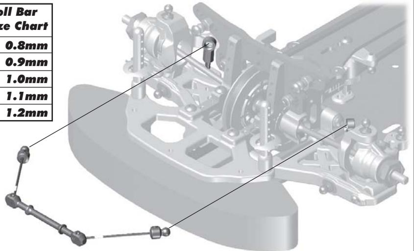
**:: Anti-Roll Bars Build / Install - Bag I-II - Step 3**
