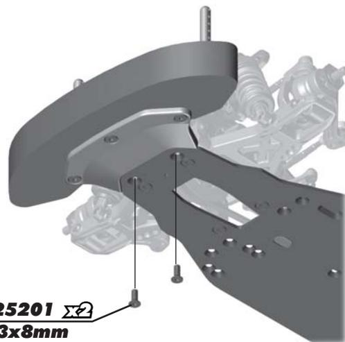
**:: Pivoting Body Mounts Install - Bag H - Step 1**
