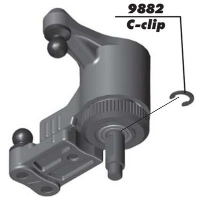
**:: Steering Bellcrank Build / Install - Bag E - Step 3**
