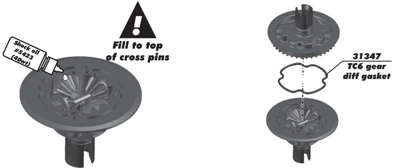
**:: Rear Gear Differential Build - Bag B-BB - Step 5**
