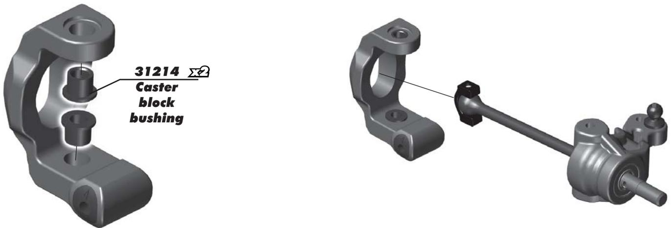
**:: Steering Block Build / Install - Bag G - Step 4**
