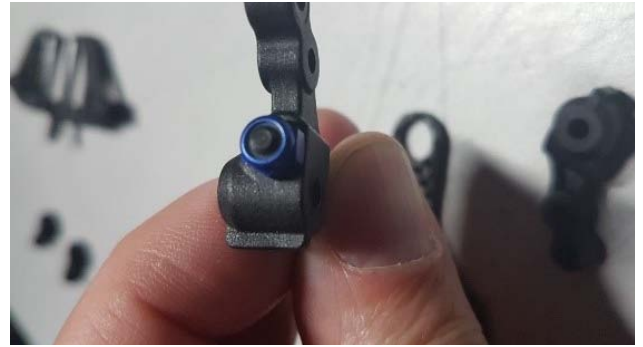
Fig 7. Ensure the flat of the nut is aligned like this to ensure it doesn't clash with the wishbone on lock.
