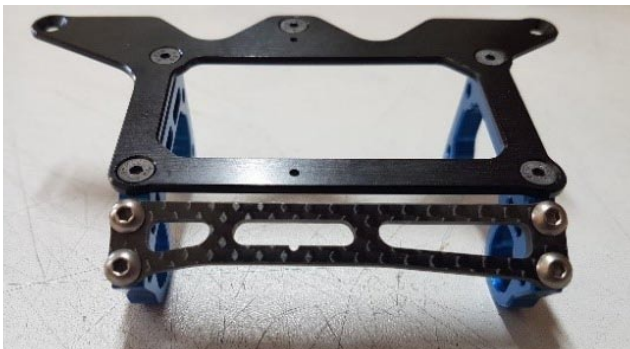
Fig 3. Note the notch cut into the carbon brace. Make sure this is aligned with the holes in the lower pod plate.
