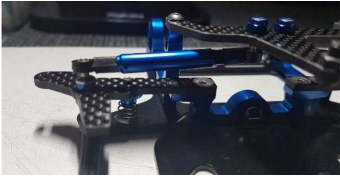
Fig 6. Note that the damper tube has been installed with the tube to the outside of the car.
