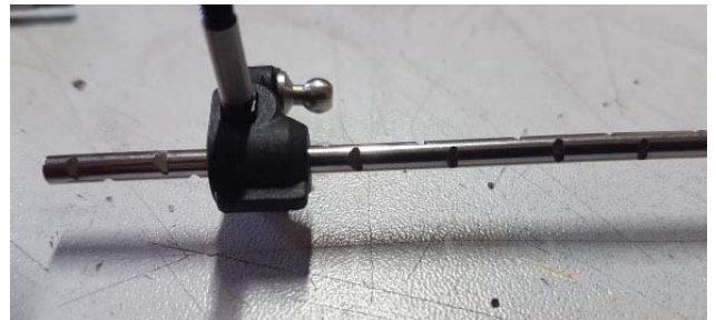
Fig 8. Run an arm reamer through the hub once the axle has been installed.
