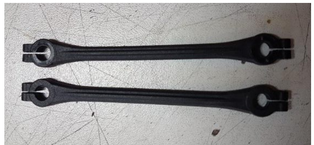
Fig 4. Note the shiny side of the side link at the top of the picture – make sure the pivot ball is installed from this side.
