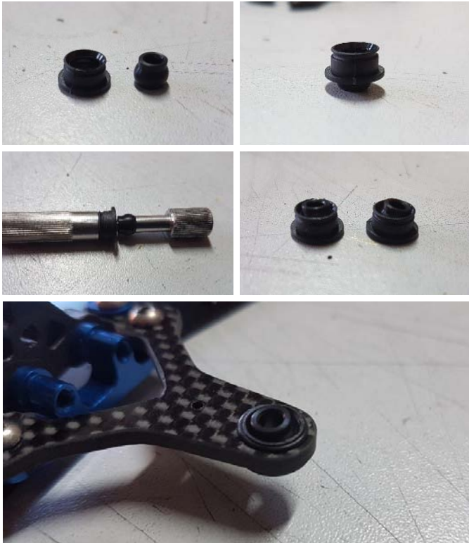
Fig 9. The correct sequence of installation and the completed front arm assembly on the car.
