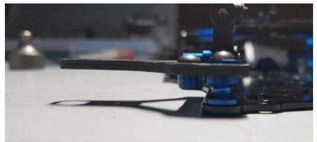
Fig 10. Note the 0.5mm spacer above the arm mounting standoff rather than below.
