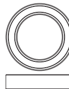
R806020 12x18x4mm Ball Bearing (4)
