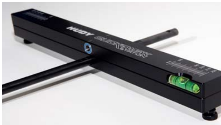
ABOVE: Using the front bubble to set the rear support horizontal, then likewise the central rod
