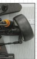
On most cars spacing the inner link forwards reduces the Ackermann effect, so that the difference in steering throw between the inside and outside wheels is reduced.
